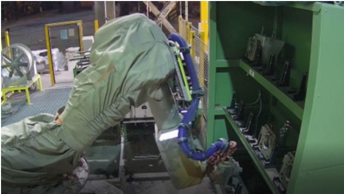
Fig. 2 The tool warehouse of the RoboHarsh workstation
