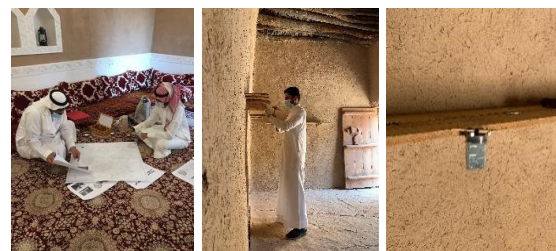
Figure 1: HOBO loggers installed in vernacular houses
