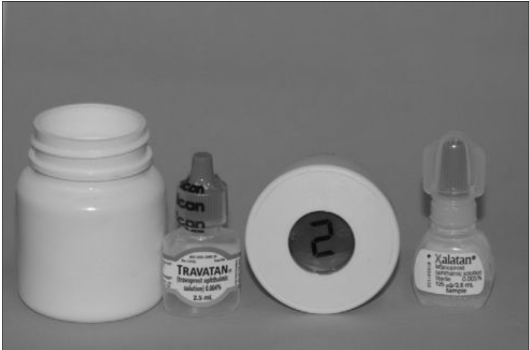
Figure 2.5: The picture above displays a standard pharmaceutical prostaglandin bottle with MEMS cap which used to measure adherence of eye drop electronically. The '2' on the cap implies two usages within 24hrs [134].
