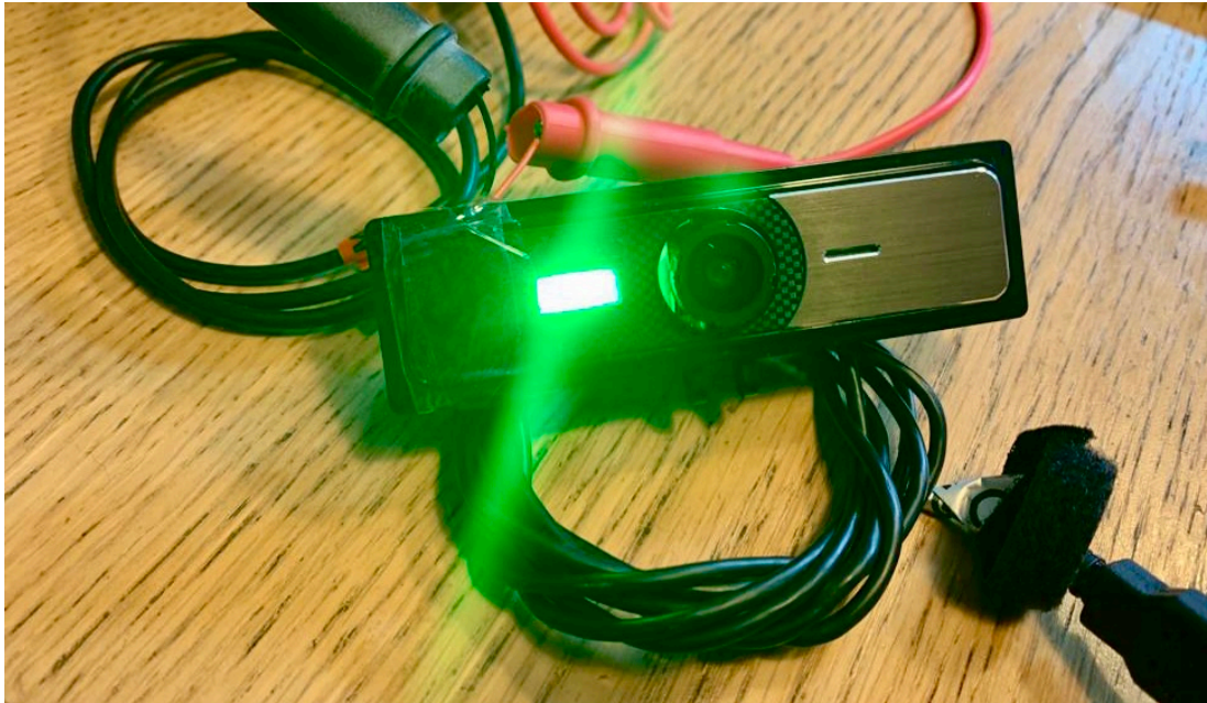
Figure 7.16: LED incorporated into the webcam.
