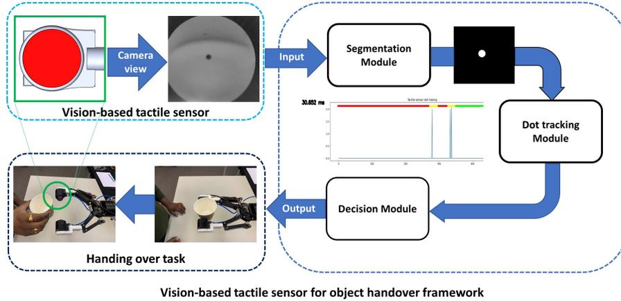
Fig. 1. Vision-based tactile sensor for handover framework
