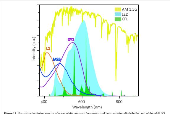
**Figure 13.** Normalized emission spectra of warm white compact fluorescent and light-emitting-diode bulbs, and of the AM1.5G solar spectrum with absorption overlay of prominent indoor dyes: L1, XY1 and MS5. LED: light-emitting diode. CFL: compact fluorescent lamp.
