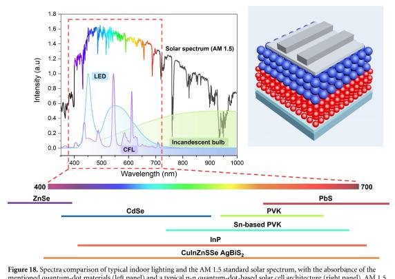
**Figure 18.** Spectra comparison of typical indoor lighting and the AM 1.5 standard solar spectrum, with the absorbance of the mentioned quantum-dot materials (left panel) and a typical p-n quantum-dot-based solar cell architecture (right panel). AM 1.5 data is from National Renewable Energy Laboratory (NREL), and indoor lighting spectra are from National Centers for Environmental Information (NCEI) and normalized CFL: compact fluorescent. PVK: perovskite.
