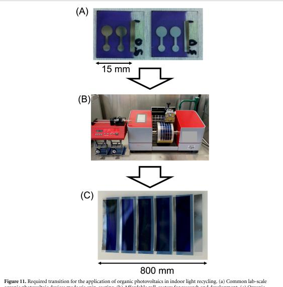
organic photovoltaic devices made via spin-coating. (b) Affordable roll-coaters for research and development. (c) Organic photovoltaic module (5 cell) made via roll-coating using halogen-free solvents with current photoactive and interlayer materials. Photos original from Welch lab.
