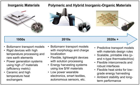
Figure 70. Evolution of thermoelectric materials and applications from high-temperature inorganic devices to flexible energy harvesters that leverage organic materials for the Internet of Things.
