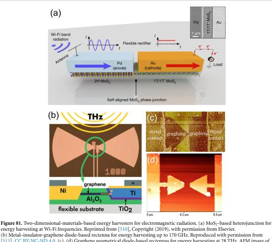
(b) Metal-insulator-graphene diode-based rectenna for energy harvesting up to 170 GHz. Reproduced with permission from [511]. CC BY-NC-ND 4.0. (c), (d) Graphene geometrical diode-based rectennas for energy harvesting at 28 THz. AFM image of the diode (c) and the antenna (d). Reproduced from [512]. © IOP Publishing Ltd. All rights reserved.
