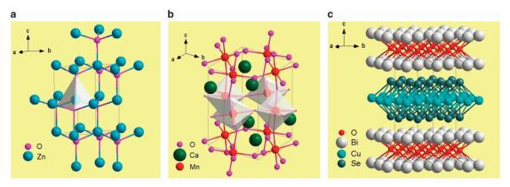
**Figure 56.** The crystal structure of (a) simple wurtzite oxide-based materials: ZnO (P63mc), (b) perovskite oxides: CaMnO<sub>3</sub> (Pbnm) and (c) layered oxides: BiCuSeO (P4/nmm).
