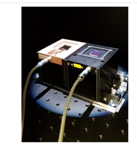
**Figure 19.** For current vs. voltage measurements of indoor photovoltaics, a calibrated reference cell (right) is placed next to the indoor photovoltaic cell (left) and used to measure and adjust the effective irradiance of the incident light-emitting-diode illumination. The objective is to measure and report the electrical performance parameters of indoor photovoltaics under a pre-defined reporting condition.
