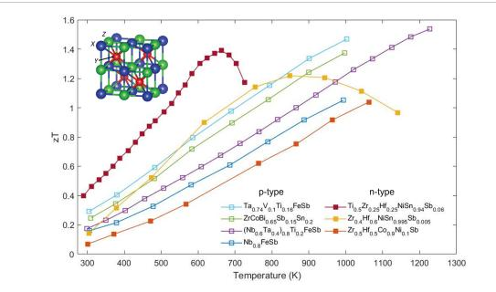
**Figure 50.** *ZT* of highest performing p-type and n-type half-Heusler alloys from Quinn *et al* [303] with an insert showing the half-Heusler structure adapted from Brod *et al.* Reproduced from [303]. CC BY 3.0. [305] John Wiley & Sons. © 2022 Wiley-VCH GmbH.
