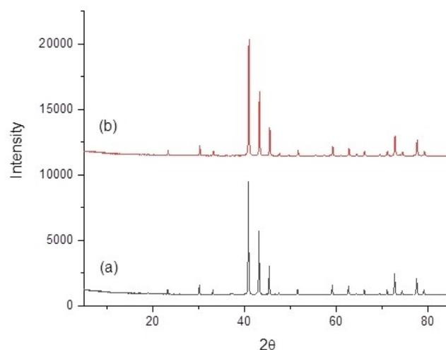
**Figure 7.** XRD patterns of  $\text{Ni}_2\text{Mo}_{2.8}\text{W}_{0.2}\text{N}$ : (a) pre-reaction and (b) post-reaction under 3:1  $\text{H}_2/\text{Ar}$  at  $400^\circ\text{C}$ – $700^\circ\text{C}$ .
