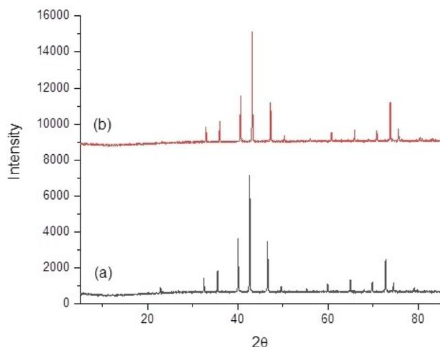
**Figure 5.** XRD patterns of  $\text{Co}_3\text{Mo}_{2.6}\text{W}_{0.4}\text{N}$ : (a) pre-reaction and (b) post-reaction under 3:1  $\text{H}_2/\text{Ar}$  at  $400^\circ\text{C}$ – $700^\circ\text{C}$ . A shift in the position of the reflections to higher  $2\theta$  with respect to pattern (a) corresponding to loss of lattice N can be seen in (b).
