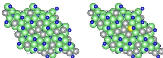
**Figure 2.** Graphic illustrating the Ni<sub>2</sub>Mo<sub>3</sub>N (111) thin film model (left) and the W-doped Ni<sub>2</sub>Mo<sub>3</sub>N (111) (Ni<sub>32</sub>Mo<sub>59</sub>WN<sub>28</sub>) thin film model (right). Note the superficial similarity of the surface structure to the W-doped Co<sub>3</sub>Mo<sub>3</sub>N model (Figure 1). Key: Ni, grey; Mo, green; W, yellow; N, blue.
