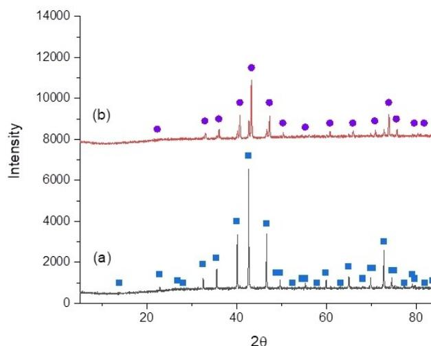
**Figure 4.** XRD patterns of  $\text{Co}_3\text{Mo}_3\text{N}$ : (a) pre-reaction and (b) post-reaction under 3:1  $\text{H}_2/\text{Ar}$  at  $400^\circ\text{C}$ – $700^\circ\text{C}$ . (□)  $\text{Co}_3\text{Mo}_3\text{N}$  and (●)  $\text{Co}_6\text{Mo}_6\text{N}$ .
