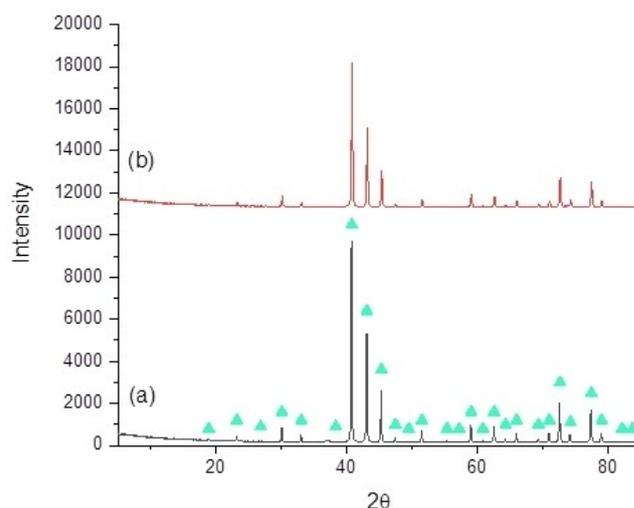
**Figure 6.** XRD patterns of  $\text{Ni}_2\text{Mo}_3\text{N}$ : (a) pre-reaction and (b) post-reaction under 3:1  $\text{H}_2/\text{Ar}$  at  $400^\circ\text{C}$ – $700^\circ\text{C}$ . ( $\Delta$ )  $\text{Ni}_2\text{Mo}_3\text{N}$ .
