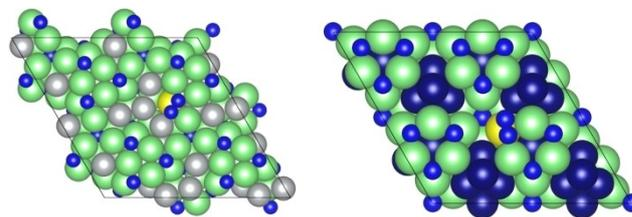
**Figure 9.** Graphic illustrating the adsorption of  $\text{N}_2$  on a surface lattice N vacancy site for W-doped  $\text{Ni}_2\text{Mo}_3\text{N}$  ( $\text{Ni}_{32}\text{Mo}_{59}\text{WN}_{28}$ ) (left) and W-doped  $\text{Co}_3\text{Mo}_3\text{N}$  ( $\text{Co}_{52}\text{Mo}_{47}\text{WN}_{28}$ ) (right). Key: Ni, grey; Co, dark blue; Mo, green; W, yellow; N, pale blue.
