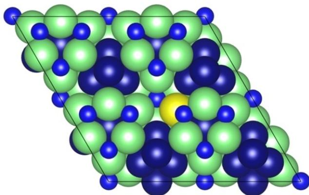
**Figure 1.** Graphic illustrating the model W-doped Co<sub>3</sub>Mo<sub>3</sub>N (Co<sub>52</sub>Mo<sub>47</sub>WN<sub>28</sub>) surface. Key: Co, dark blue; Mo, green; W, yellow; N, pale blue.
