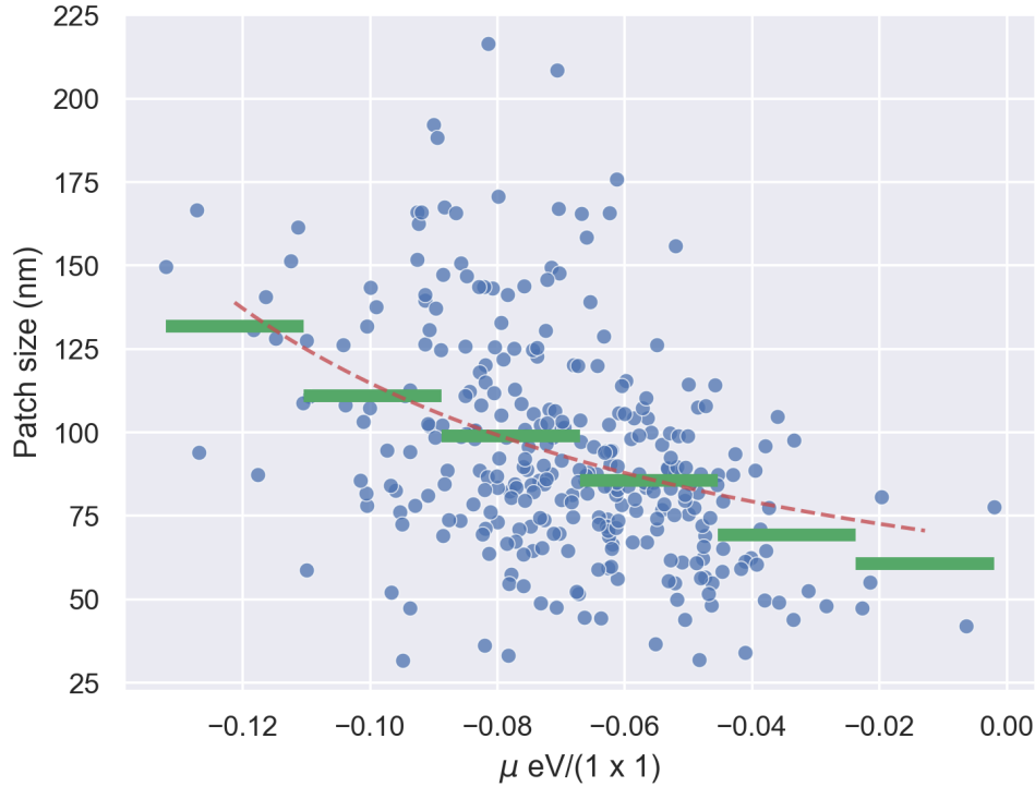
Figure 4.7: Patch size against chemical potential upon transformation. The final size of each patch before transformation is represented with a blue dot. The average radius size (green bars) is calculated for chemical potential steps of \Delta\mu_{Ga} = 0.015 \text{ eV} and the fit from Equation 4.5 is shown with the red dashed line.
