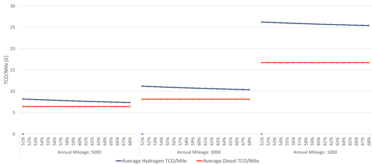
Figure 4.8: TCO/Mile of average hydrogen RCV with increasing efficiency vs TCO/Mile of average diesel RCV
