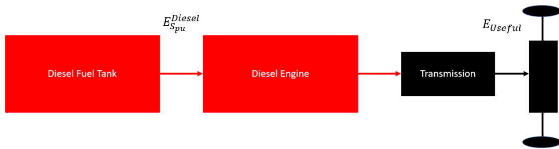
Figure 4.1: A diesel vehicle's components and energy flows
