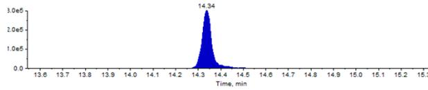
A blank methanol injection showing no peak/noise. Integration of the window (14.3-14.4) shows area above 2000
