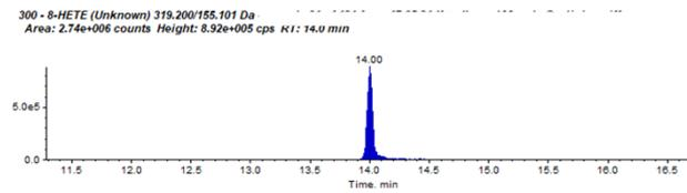
Three blank methanol injections showing no peak. Integration of the window (13.95-14.08) all show areas above 2000
