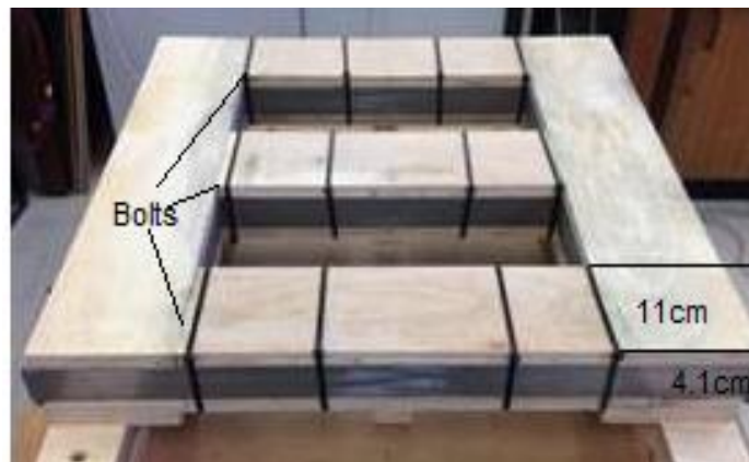
Figure 4- 1 Transformer under study
