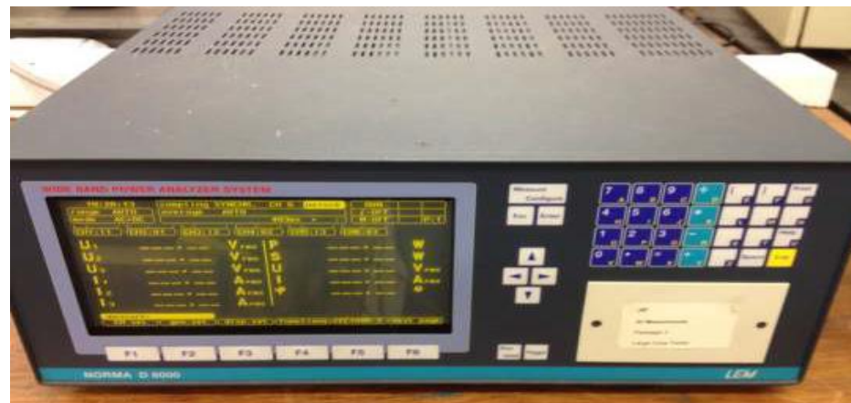
Figure 3 Power analyzer system
