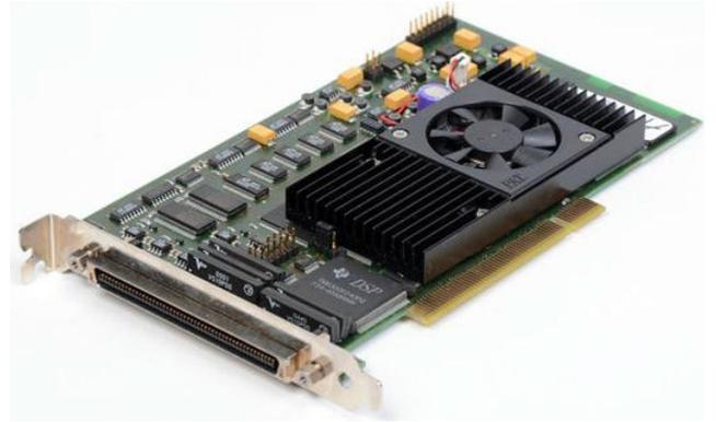
FIGURE 20. Dspace DS1104 research and development controller board.
