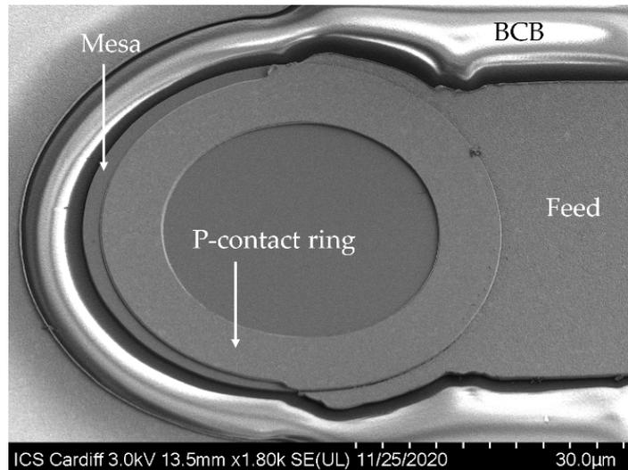
Figure 4.1: SEM image of BCB-planarised standard VCSEL device. The mesa is fully isolated by an open-area etch. BCB is used to facilitate a planar deposition of the ring-contact and feed metal.
