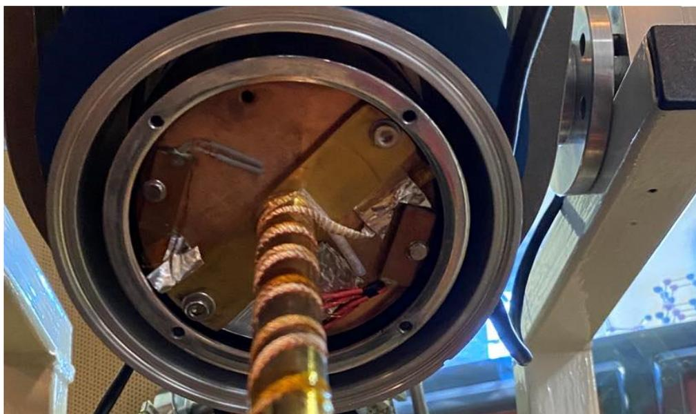
*Figure 35: Second cold plate – Heater and thermometer are mounted in the copper blocks for thermal contact with the plate and cold finger.*
