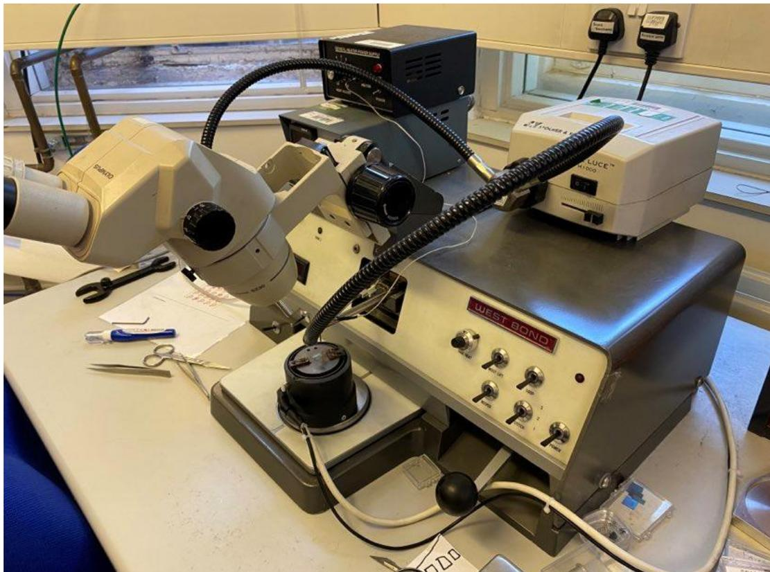
Figure 33: West Bond wire bonder used for gold-to-gold contacts.
