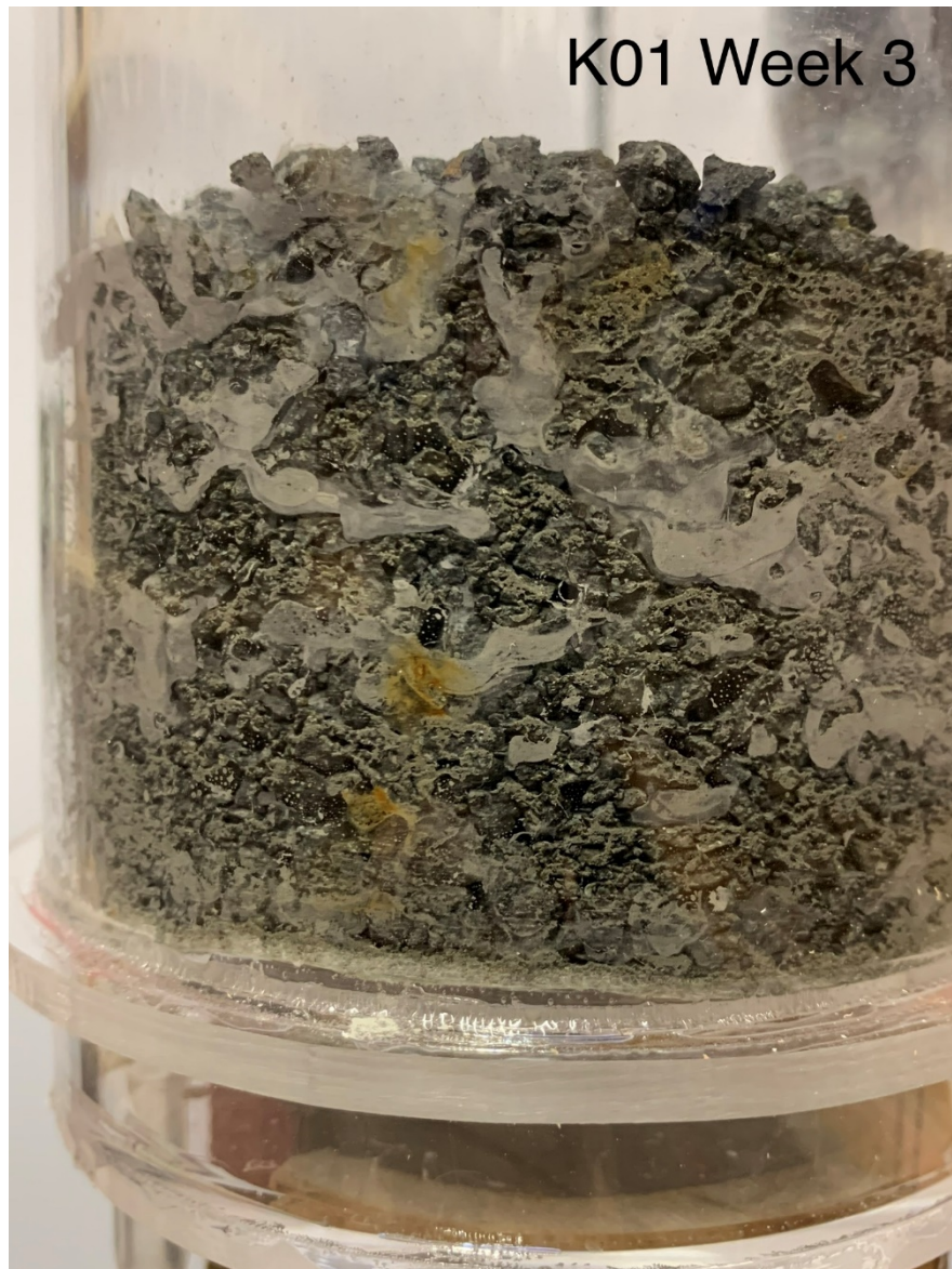
Figure A22.4 - Cell K01 image taken outside of cell in week 3. Potential signs of oxidation of iron bearing minerals.
