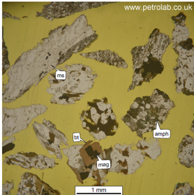
Figure A3.39 - Sample GCL0100- A08-Post - Cross polarised light image of previous photo
