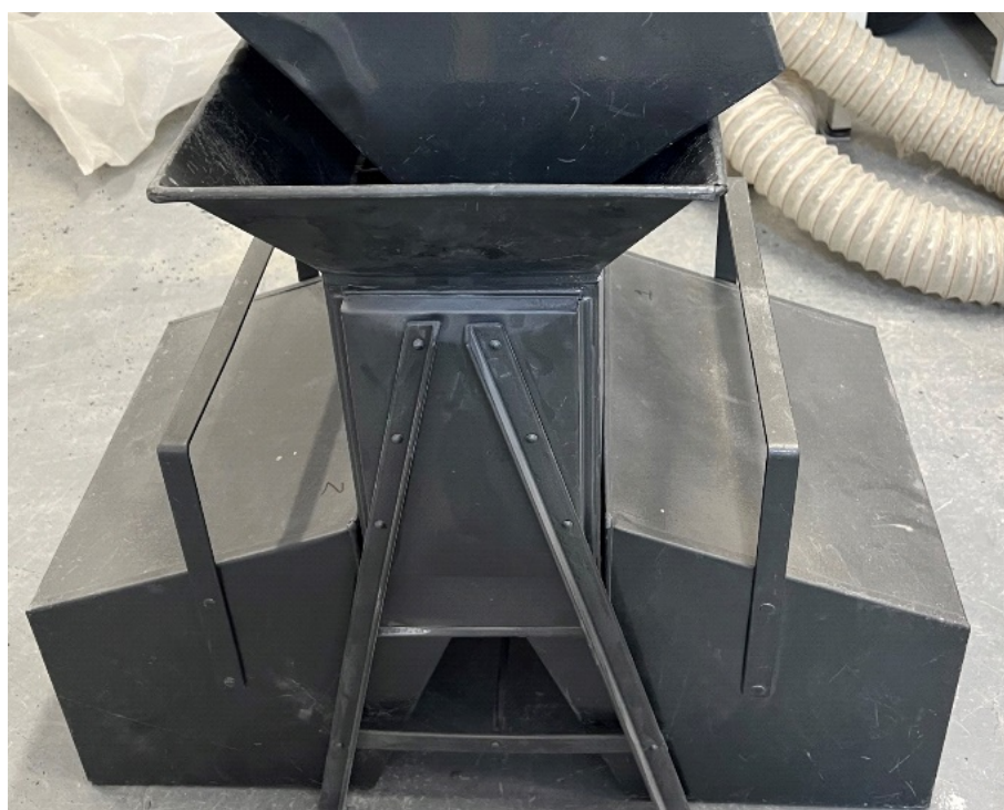
Figure 22 - Riffle box splitter used in stage 1 splitting.
