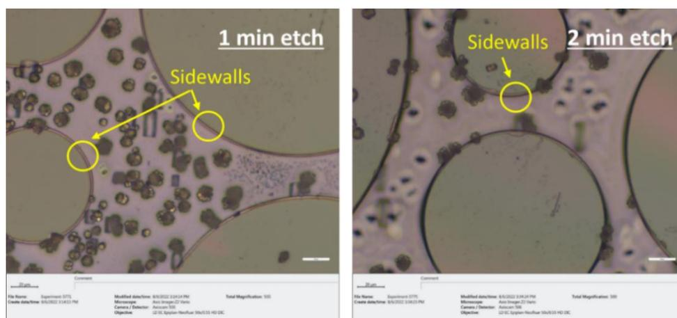
Figure 7.12: Optical micrographs of the etched InAs/GaSb T2SL samples using a combination of recipes SD1 and SA.
