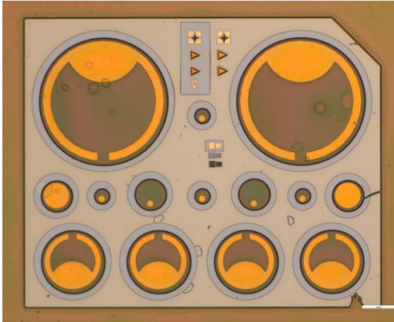
Figure 6.17: Optical micrograph of a MWIR InAs/GaSb T2SL fabricated device with different mesa diameters ranging from 440 to 90  $\mu\text{m}$  utilising the dry + wet etch technique and surface protection with the photoresist (Sample C3).
