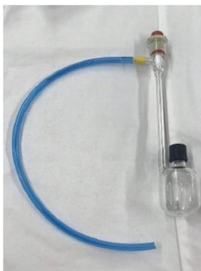
**Figure 2.1:** a Colaver reactor® for the catalyst testing.
