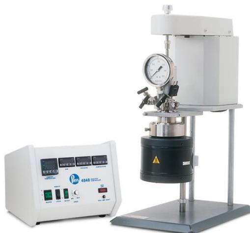
**Figure 2.2:** 50ml stainless-steel autoclave reactor by Parr Instruments.
