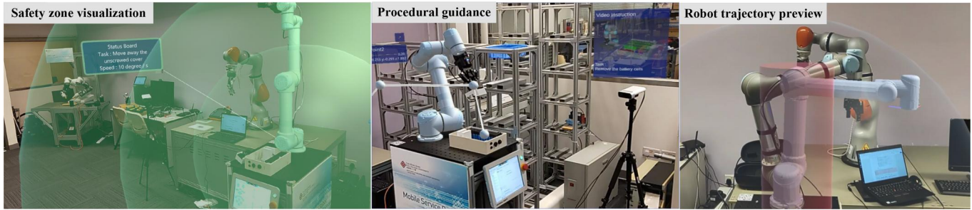
Figure 7. System demonstration of MR-based information support and trajectory preview.
