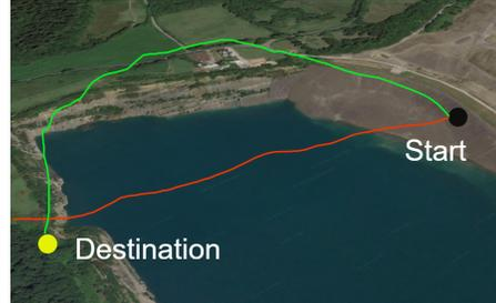
Fig. 1: A drone travels from the start to the destination, crossing a lake. The red trajectory, although shorter, lacks reliable visual features for pose tracking. In contrast, the longer green trajectory enhances visual odometry performance by maximising feature quality over terrain, houses, etc.
