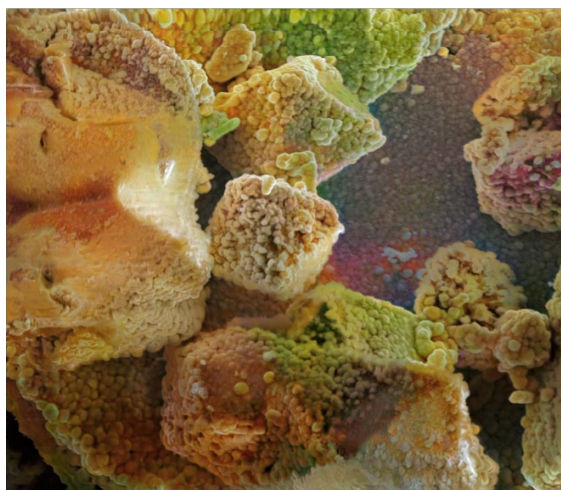
FIGURE 9.1: It is the SEM image (polygon shaped) of a paddle wheel-based bimetallic ZnCuBTC metal-organic framework containing an antiferromagnetically coupled S = 1 spin state Cu(II)-Cu(II) dimers - portrayed as a Coral reef - Underwater artwork
