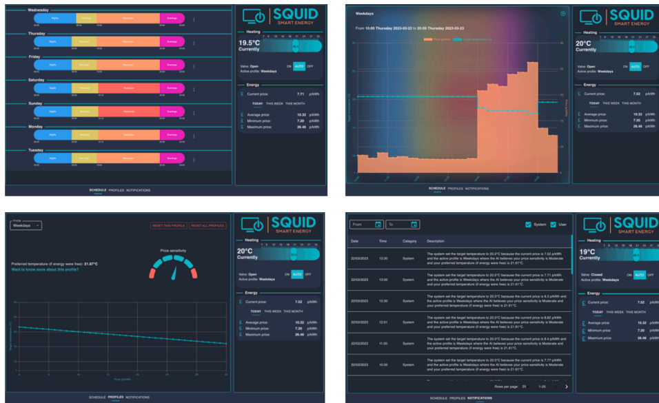
Fig. 2. Squid. Top left: Heating profile scheduler; Top right: AI temperature schedule visualisation; Bottom left: AI summary and gauge visualisation. Bottom right: Notifications log.
