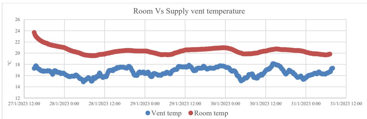
Figure 12 Comparison of room and supply vent temperature for the experiment
