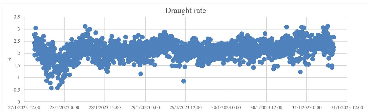
Figure 11 Draught rate calculated using EN ISO 7730 guidelines
