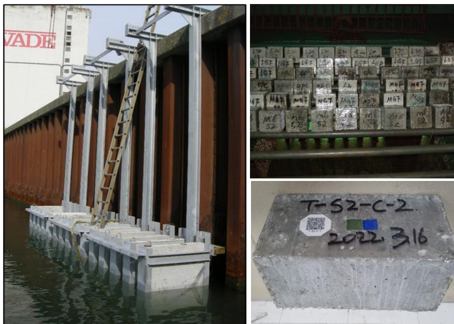
Figure 3: Large-sized specimens (0.2mx1mx2m) from exposure site at Rødbyhavn, Denmark (left) and small-sized specimens (100mm cubes) in Zhanjiang exposure site, China (upper right), and a label tag on exposed specimen (down right). Courtesy of Dr. Henrik Erndahl Sørensen and Dr. Xiong Jianbo (CCCC).
