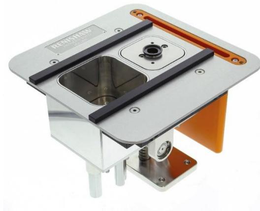
Figure 3.1: Renishaw Reduced Build Volume (RBV) system, from [151].
