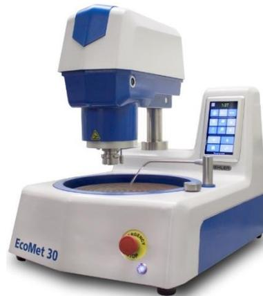
Figure 3.6: Buehler EcoMet 30 grinder polisher machine, from [156].
