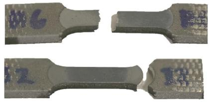
Figure 6.11: Example of sample failure (top) within the gauge length, and (bottom) failure at edge of polished region.
