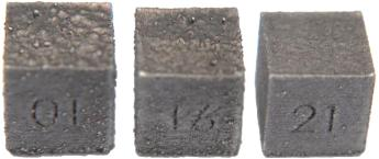
Figure 2.17: Typical surfaces from AM Aluminium.
