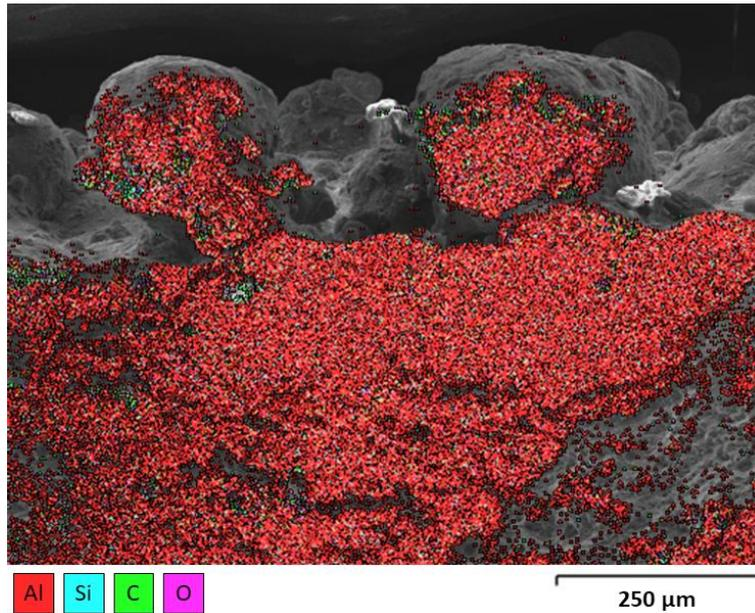
Figure 7.8: EDX composition map from As Built condition LCF sample.
