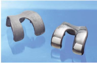
Figure 2.12: Example of AM prosthetic knee joint, in the as built condition (Left) and after laser polishing (right). From [66].
