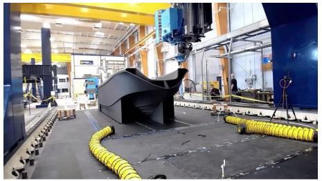
Figure 2.1: Additively manufactured polymer boat hull produced by University of Maine [18], similar in concept and execution as the device described by Leinster [16].
