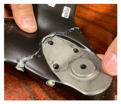
*Figure 2.16: Australian Olympic cycling team AM Titanium component failure, attributed in part to improperly defined loading conditions during design, accelerating the onset of fatigue cracking. From* [85].
