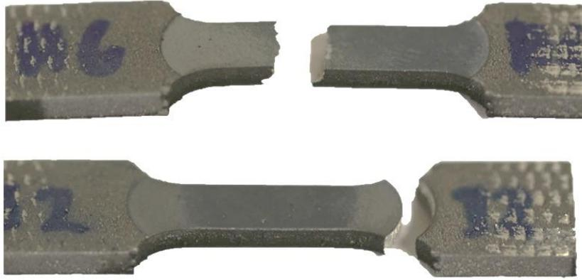
Figure 6.11: Example of sample failure (top) within the gauge length, and (bottom) failure at edge of polished region.
