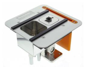
Figure 3.1: Renishaw Reduced Build Volume (RBV) system, from [151].
