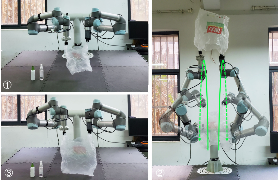
Figure 2.6: ShakingBot using the physical capacities of the bag in its favour to open it in three steps (Gu et al. 2024). First the robot locates the bag handles and then uses the material’s properties to maintain its shape in order to complete the task.
