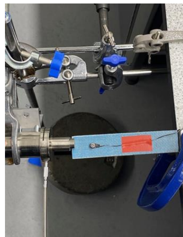
Figure 1. Simulation of displacement of FlaxPP composite sample while undergoing vibration
