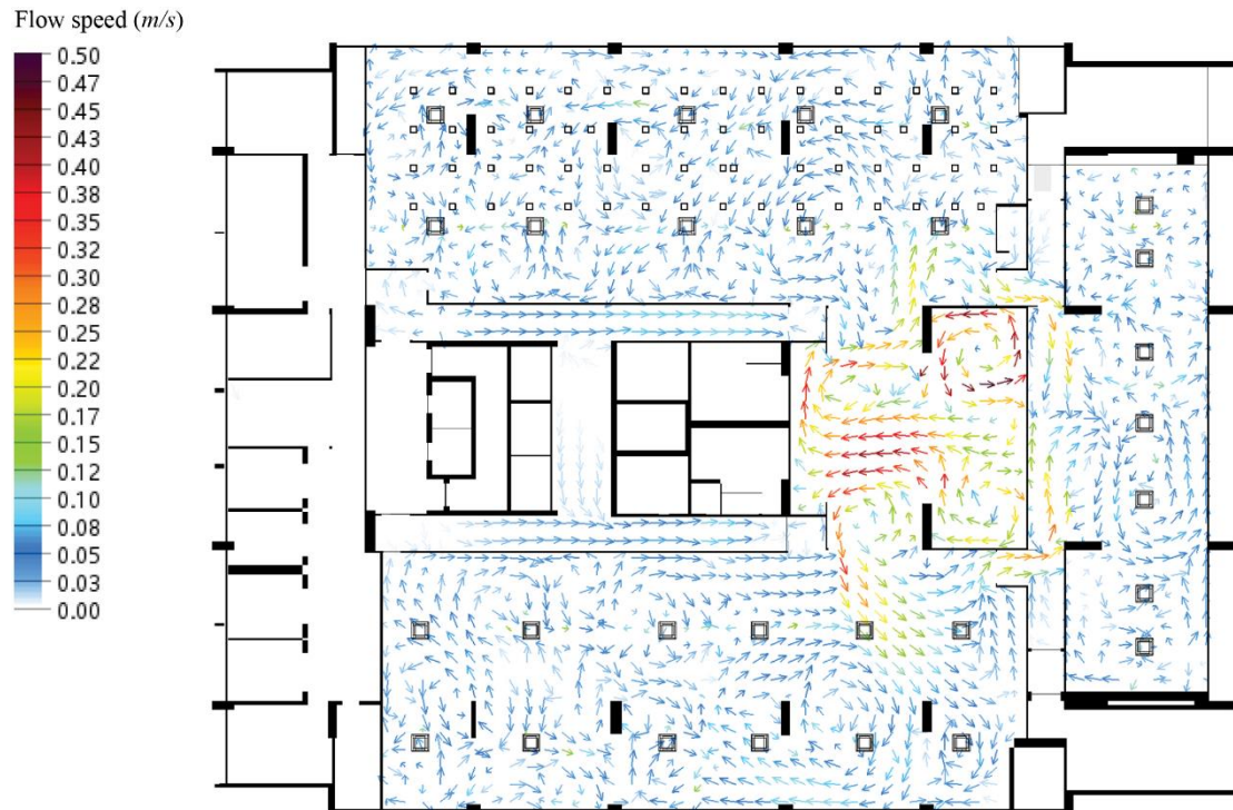
Fig. A.5. The predicted velocity field at a height of 1.5m.
