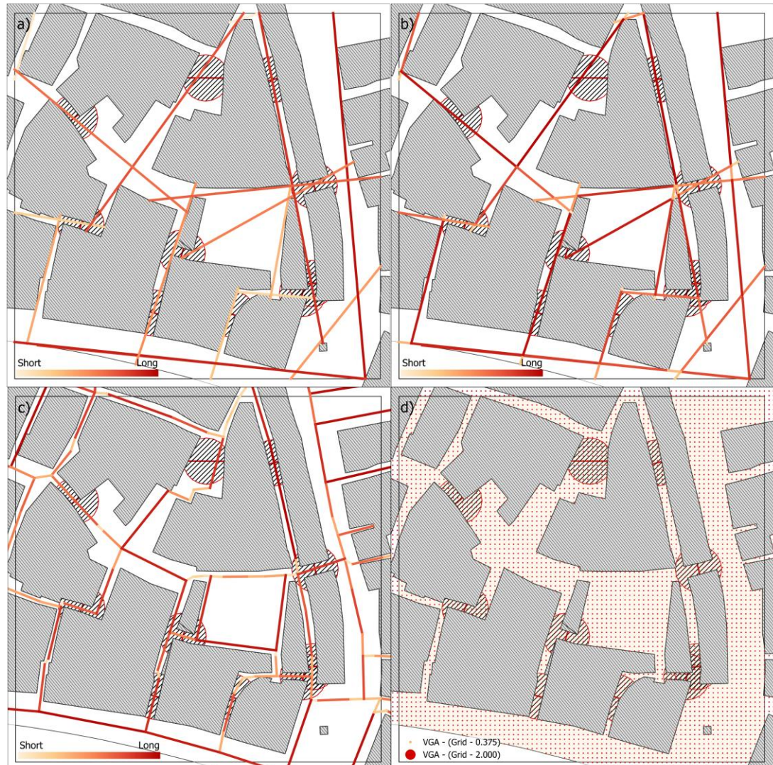
Figure 3. Grids for the analyses: categorized by length – lines for AA (a), segments for ASA (b), RCL segments for ASA (c); and categorized by size – vertices for VGA (d).
