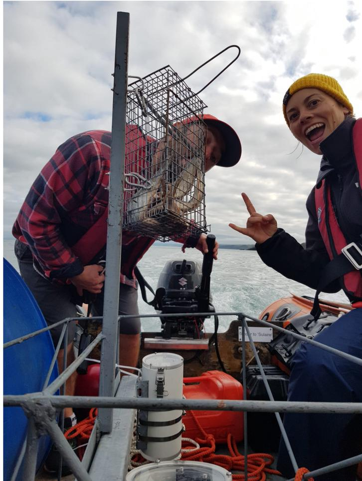
**Figure 1.4 Stereo baited remote underwater video stations (BRUVS), Cardigan Bay. The tether point for the rope can be seen in the bottom right of the image, such that when the BRUVS is deployed the bait arm and camera fields of view are horizontally aligned with the substrate.**
