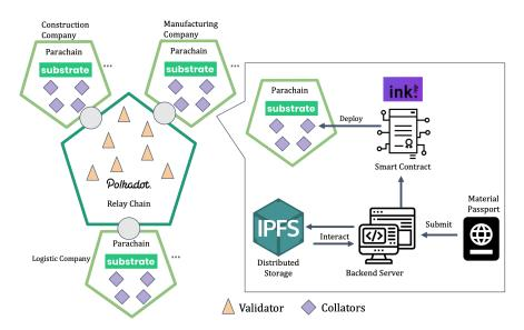
Figure 2. Multilayer blockchain architecture [8].
