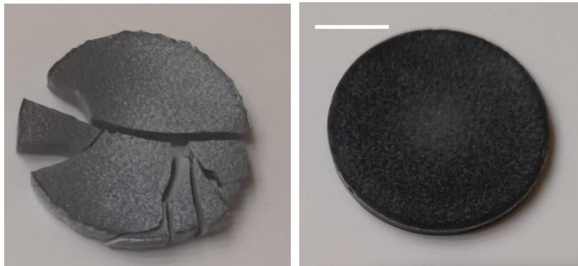
**Figure 3.18** – Photographs illustrating the comparison between sintered alumina specimens. **Left)** preliminary sintering conditions. **Right)** modified conditions using a continuous DC pulse sequence, lower pressure, and lower heating/cooling rates. Scale bar = 10 mm.
