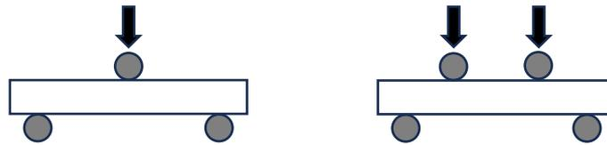
**Figure 1.5** – Illustrations of three- and four-point flexure testing. Arrows represent an applied load.
