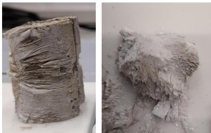
**Figure 4.7** – Images of a 40 wt.% alumina scaffold that has been drop-cast with a 0.025 wt.% suspension of  $\text{GO}_{\text{supplier}}$ . **Left)** infiltrated scaffold. **Right)** core section of the specimen that illustrates the deposition of  $\text{GO}_{\text{supplier}}$  through FD axis.
