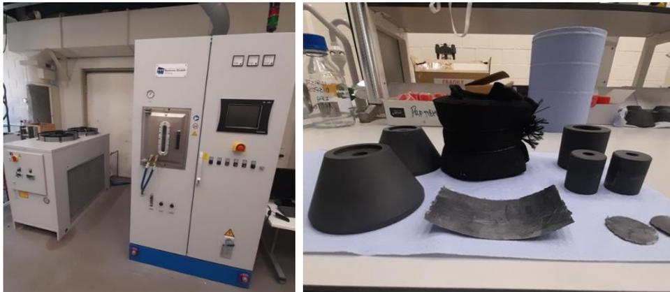
**Figure 2.7 – Left)** photograph of SPS Type HP D10-SD and chiller unit. **Right)** graphitic components used to assemble 30 mm die sets.
