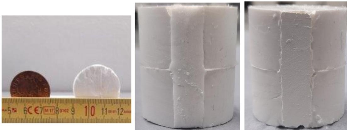
**Figure 3.8** – Photographs of alumina scaffolds after freeze-drying. **Left)** comparison of a 25 wt.% alumina scaffold with a 2 pence coin. **Middle)** view of surface that is exposed from mould. **Right)** view of surface that contacts the copper bottom inside the mould.
