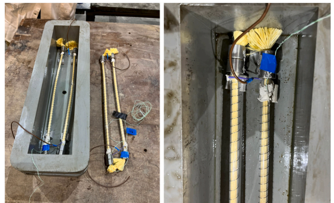
Fig. 5. Positioning of Hybrid Tendons before casting and close-up on the use of glue to keep the Kanthal wires in place.
