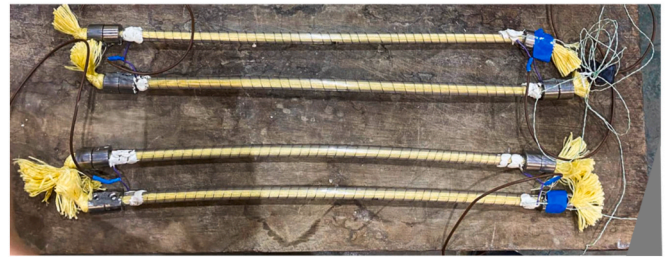
Fig. 4. Hybrid Tendons with Kanthal wires prepared to be casted within the concrete specimens.
