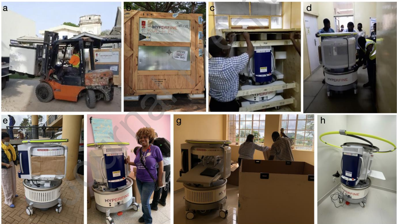
Figure 5. Pictures of Swoop arriving at a clinical cohort site. Following unloading of the scanner and accessory crate (a and b), the scanner crate is opened and protectors removed (c). The scanner can then be driven out of the grant and into the facility (d, e, and f) to its desired location. Here final set up and unpacking is performed (g) before being ready to image. From arrival to set up can take between 30-60 minutes depending on access and distance from delivery point to final scan room.
