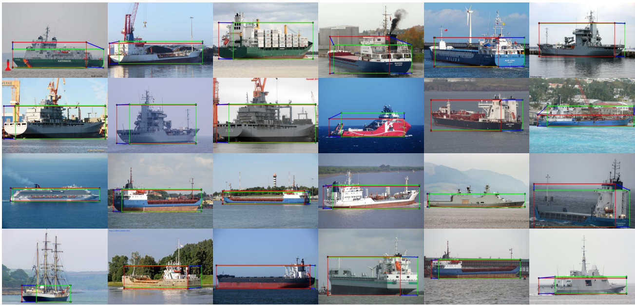
Fig. 15. Examples of landmark-based ship detection. Based on the landmarks, the bounding boxes provide information about the orientation of ships.
