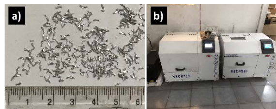
Fig. 2. a) Raw AA5083 chips, b) MECHMIN Planetary ball mill.
