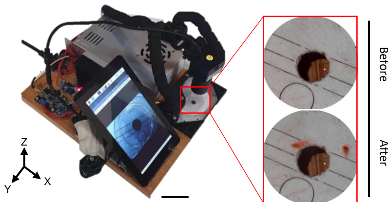
Figure 6.22. Next generation DAS system equipped with a camera, screen, and real time pellet analysis (inset). Scale bar 5 cm.
