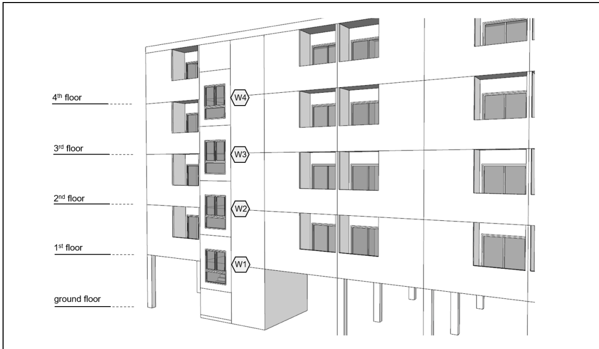
Figure 3- 6 model of a multi-storey building for collecting stack temperature, relative humidity, and air movement velocity (Source: Author)
