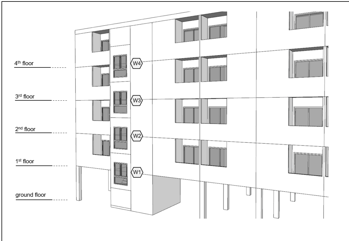
Figure 4- 1 model of a multi-storey building for collecting stack temperature, relative humidity, and air velocity (Source: Author)
