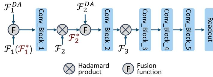
Fig. 3. Details of the CNN Decoder, where  $F_i$ ,  $i = 1, 2, 3$  denotes the saliency features from encoding phase (i.e.,  $T_i$ ,  $i = 1, 2, 3$ );  $F_i^{DA}$  and  $F_i^*$  denote the distortion-aware features from DASM, and the features that are fused with  $F_i^{DA}$  in the CNN decoder.
