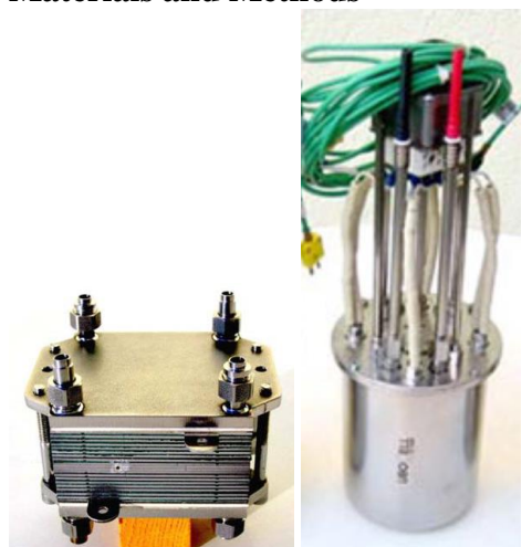
a) Stack only b) SOFC "module"
