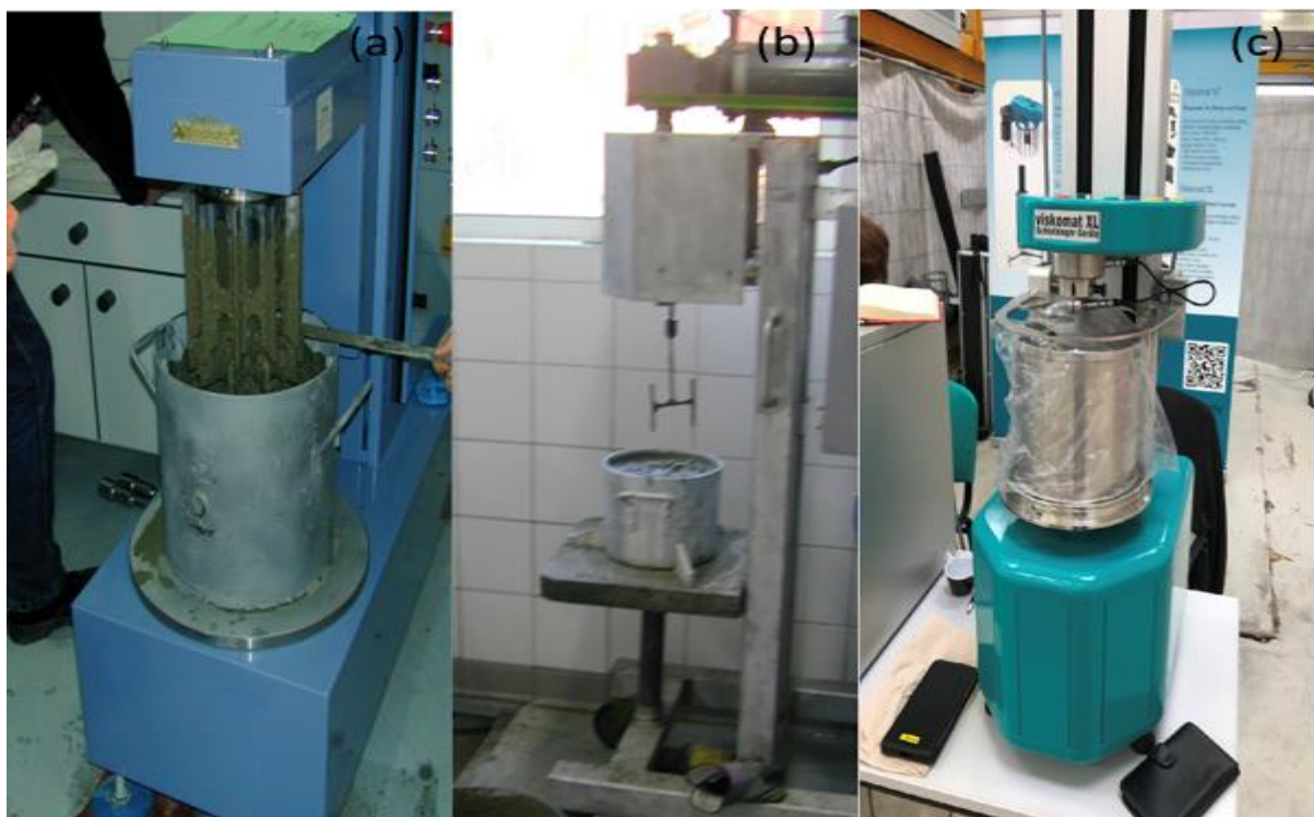
Figure 2.5 Rheometer types: (a) BML-rheometer, (b) Tattersall MK III rheometer, and (c) Vikomat XL rheometer (Sonebi and Yahia 2020)
