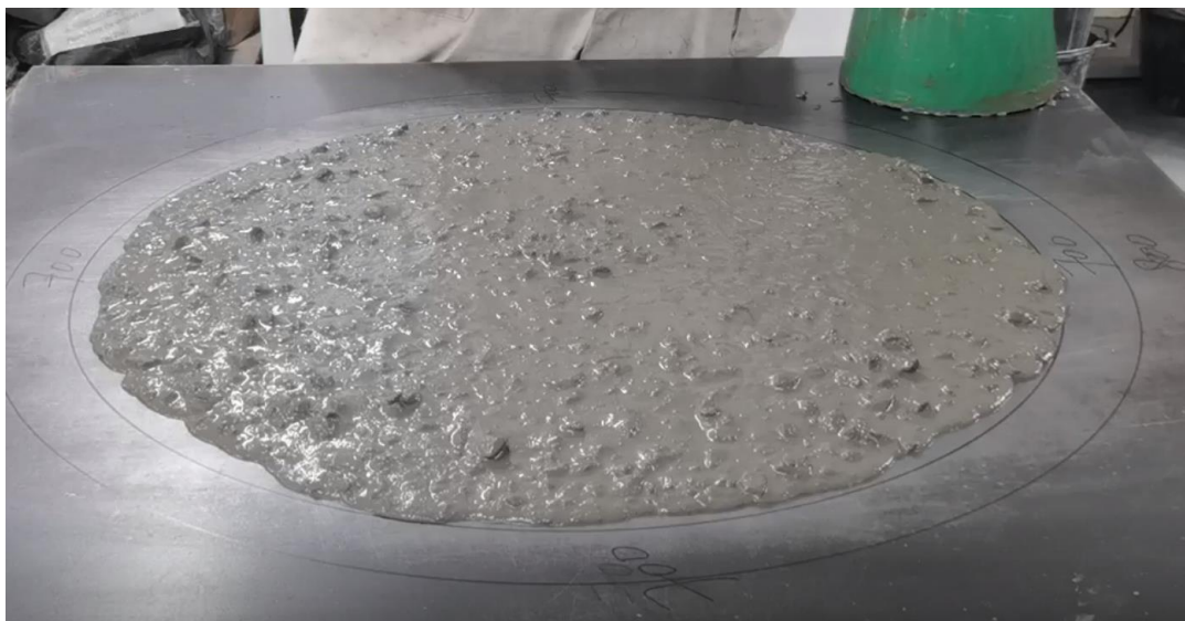
Figure 3.6 Final slump flow diameter of Mix 70C (Alshahrani et al. 2023)
