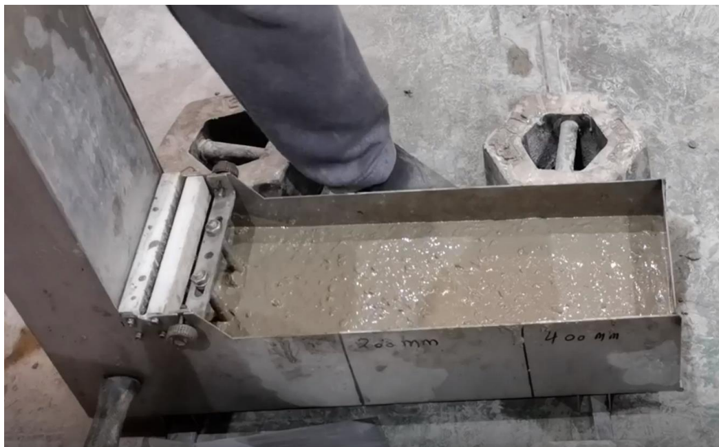
Figure 3.8 L-box test of Mix 70C (Alshahrani et al. 2023)
