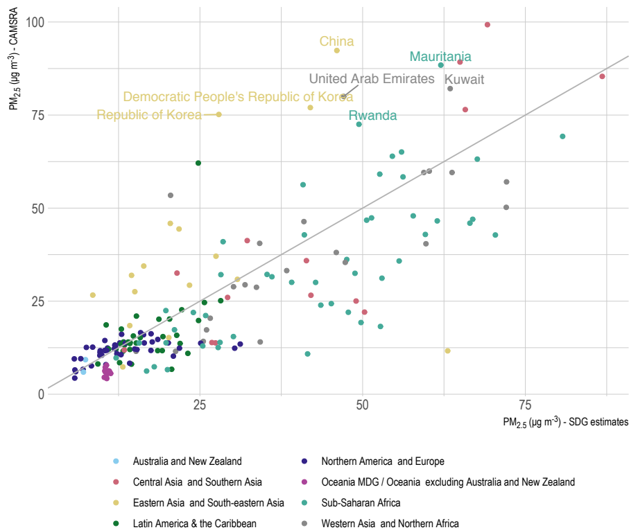
Figure 3. Comparison between the country-level population-weighted annual average of PM_{2.5} estimated by the Copernicus Atmosphere Monitoring Service multi-annual global reanalysis of atmospheric composition and SDG indicator 11.6.2 calculated using DIMAQ, by SDG region, for 2016. Grey line indicates a one-to-one relationship.
