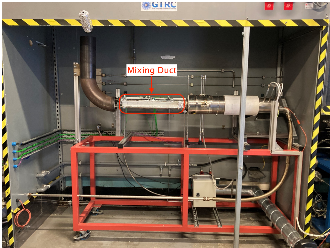
Figure 4.4.3: Annotated image of the TIMAR, highlighting the region of interest in the PIV analysis.
