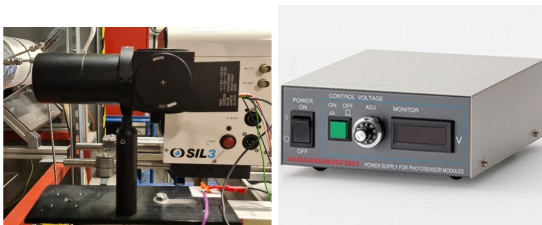
(a) Hamamatsu H9306-09b PMT set-up within the Rig Room (b) Accompanying Power Supply - Hamamatsu C7169, image reproduced from [190]
