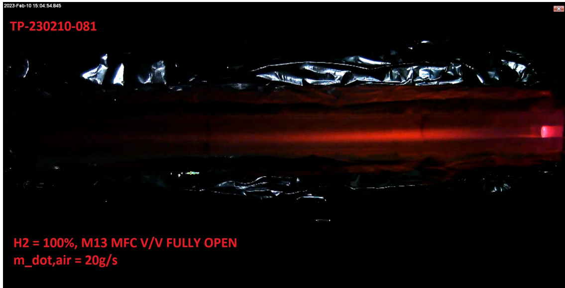
Figure 3.6.8: Image of pure hydrogen flame during commissioning, P_{therm} = 3.84kW
