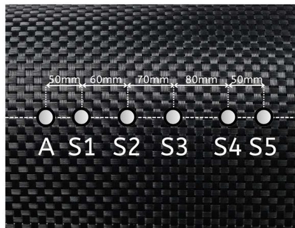
Figure 14: Linear array of actuator A and five transducers S_1 - S_5 used to acquire data for in-line signal classification on-the-edge
