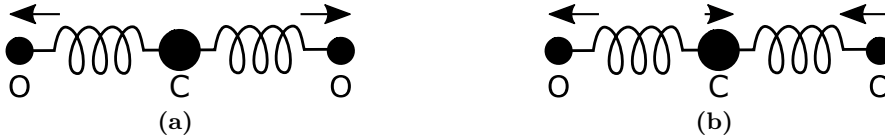
Figure 2.2: Polarizability during the oscillation must change for the mode to be Raman active. Raman active mode of carbon dioxide a) and Raman inactive mode of carbon dioxide b).
