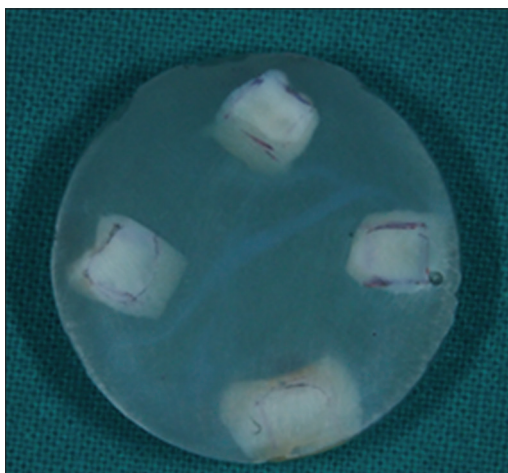
Figure 1: Enamel slabs embedded in acrylic resin (4 mm × 4 mm)
