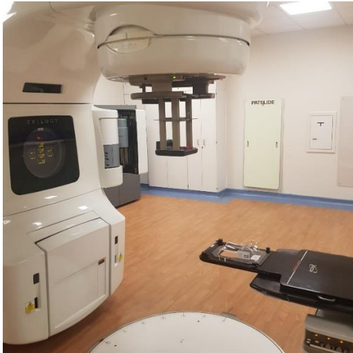
Photo 9. An applicator attached to the linac for electron treatments.
