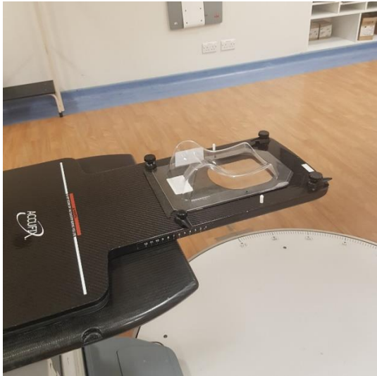
Photo 8. Position of a shim under a headrest.
