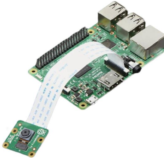
Figure 4.2 2 The image shows the physical set up for a camera with the Raspberry Pi
