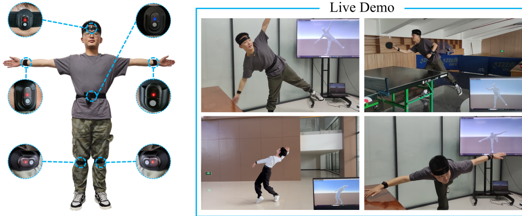
Figure 1: Left: we use only six IMUs to predict the full-body pose in real-time, which are fixed on left and right forearm, the left and right lower leg, the head, and the pelvis. Right: our system is capable of capturing a wide range of daily motions as well as challenging movements.
