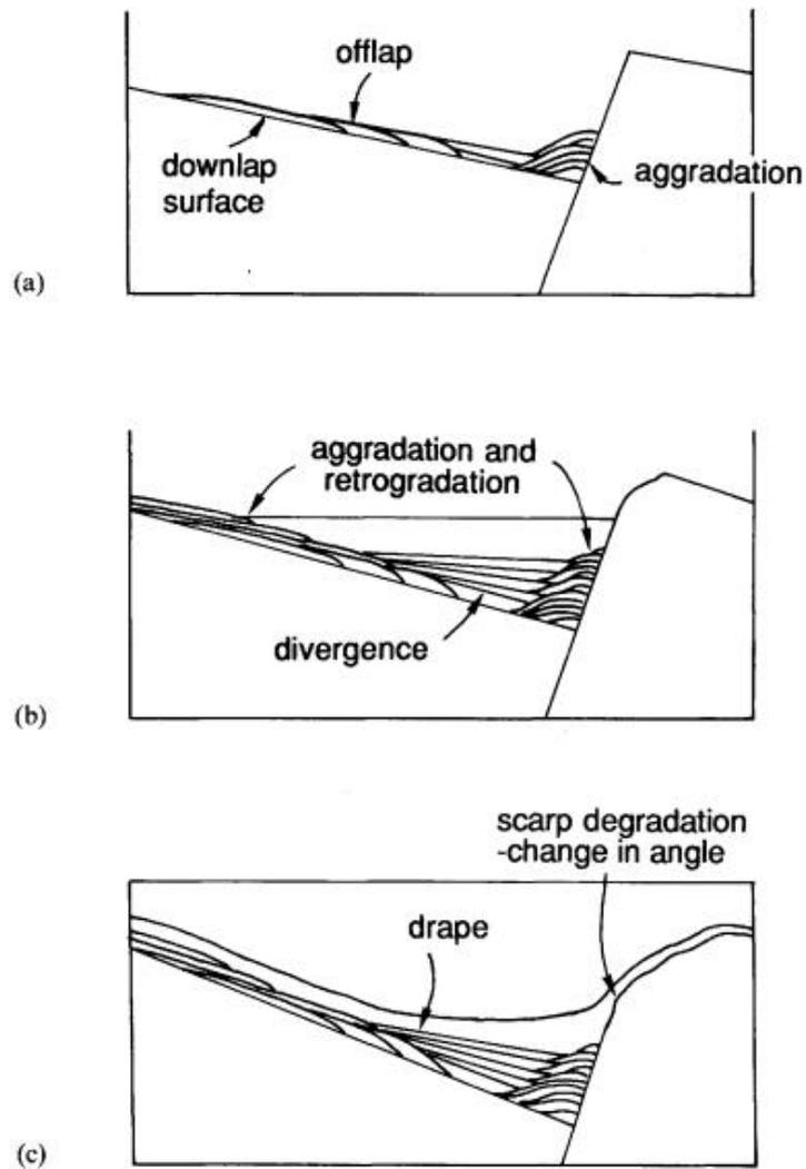
Figure 2.6: Possible reflector configurations of early, mid and late stages of rift climax systems tract. Tilting and divergence common at each stage. (a) early rift climax, (b) mid-rift climax, (c) Late rift climax. From Prosser (1993).
