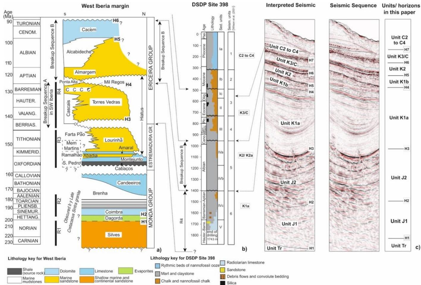
Figure 3.2: Correlation panel between interpreted seismic stratigraphic units and well data from the West Iberian Margin (Alves and Cunha, 2018) and DSDP Site 398 (Groupe Galice, 1979; Rehaut and Mauffret, 1979). See Figures 3.1b and 3.7 for detailed location of the seismic section and DSDP Site 398. Interpreted seismic horizons (Hn) are overlain on the assumed West Iberian margin equivalents.
