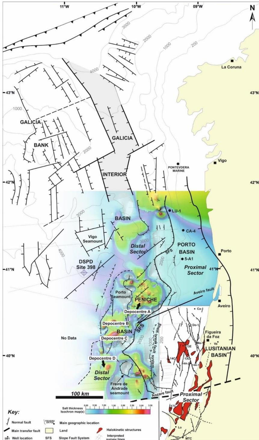
Figure 3.8: Salt thickness map in TWTT, from Horizons H1 to H2, overlain by structural elements from Alves et al. (2006) and Murillas et al. (1990). Also shown is the interpreted seismic grid. Inset map is taken from Alves (2002) highlighting halokinetic structures mapped east of the study area, in the Lusitanian Basin.
