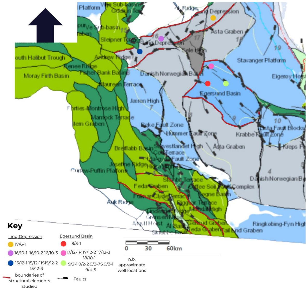
Figure 4.10: Geological Map of the Norwegian Sector of the North Sea delineating various structural elements. The map displays the Ling Depression, Egersund Basin, and Feda Graben as distinguished by red lines. Approximate locations of exploration wells are marked with coloured dots, each labelled with the corresponding well identification numbers. Adapted from Norwegian Petroleum Directorate, 2023. FactMaps [Online]. [Accessed 27 November 2023]
