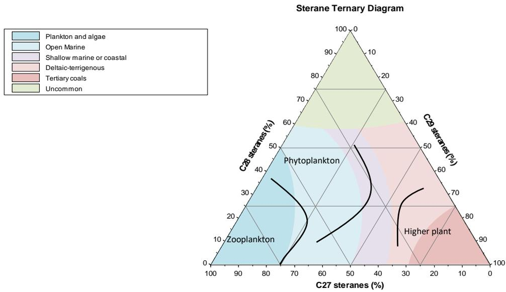
Figure 4.7: Ternary plot (Author's own) of the distributions of C27-, C28-, C29- sterol homologs used to differentiate depositional environments based on the characteristic associations of contributing organisms.
