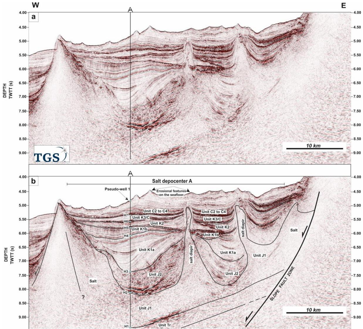
Figure 3.5: a) Uninterpreted E-W section, and b) corresponding interpretation of a seismic profile acquired 50 km southwest of the Porto Seamount. Note the developed diapirs, the clear base of salt and apparent formation of bowl-shaped depocentres during the Early Cretaceous rift 4 (Unit K1). See Figure 3.1b for location. Location of pseudo-well 1 (PW1) shown in this figure.
