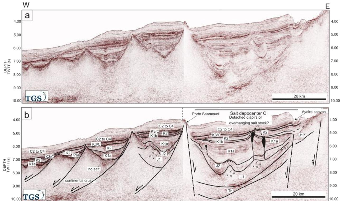
Figure 3.4: a) Uninterpreted composite line b) Interpreted seismic profile of composite line (location shown above). Note structure of Peniche Basin and adjacent deep margin area. Upper Cretaceous Unit K1 is widespread along the margin. Note the disappearance of salt west into the deep margin area. TWTT = Two-way travel time.
