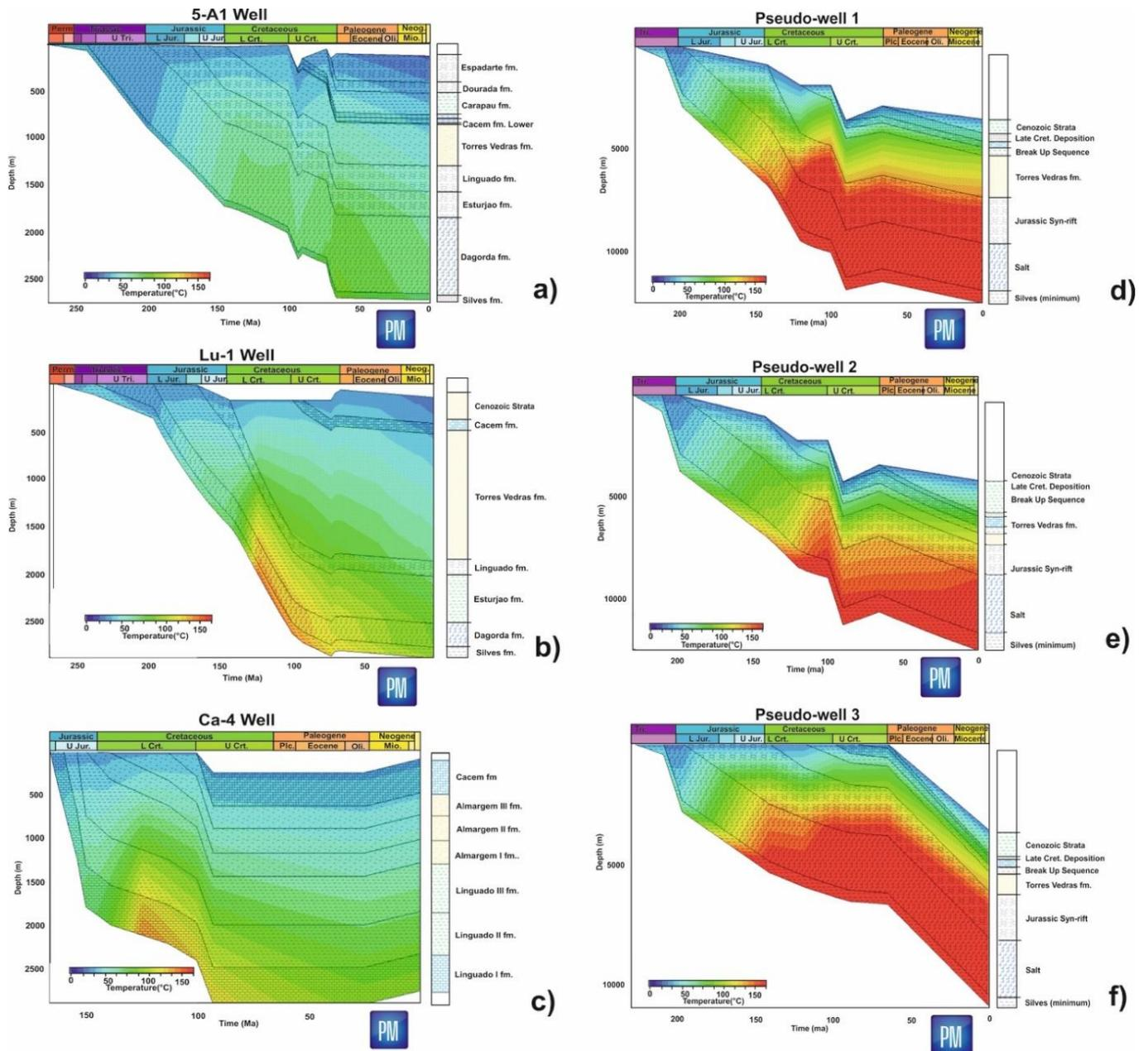
Figure 3.9: a) Thermal subsidence curve for well 5A-1. b) Thermal subsidence curve for well Lu-1. c) Thermal subsidence curve for well Ca-4. All wells located on the continental shelf. d) Thermal subsidence curve for pseudo-well 1, e) Thermal subsidence curve for pseudo-well 2, f) Thermal subsidence curve for pseudo-well 3. Pseudo-wells are located in continental-slope basins to the west of the Lusitanian and Porto Basins. (Locations of pseudo-wells are shown in Figures 3.1b.
