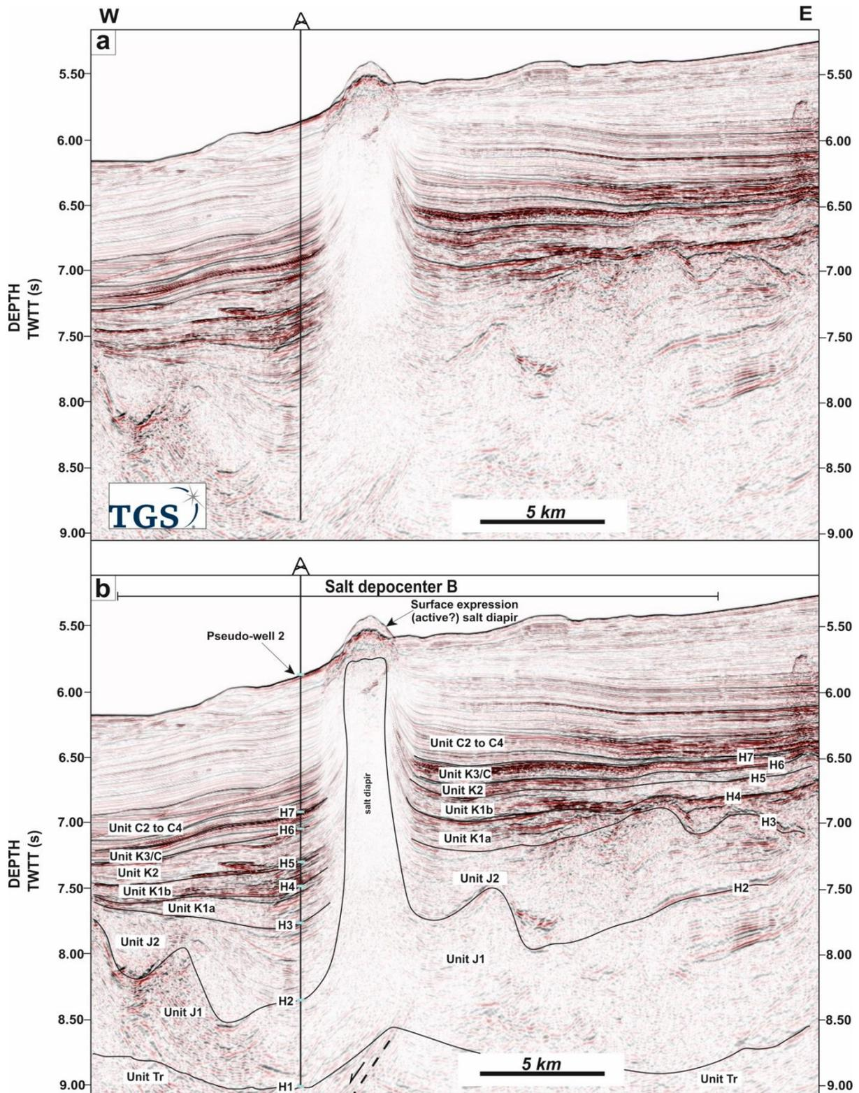
Figure 3.6: a) Uninterpreted E-W section, and b) corresponding interpretation of a E-W seismic profile located to the west of the Porto Basin. See Figure 3.1b for location. Note the surface expression of a developed salt diapir. The location of pseudo-well 2 (PW2) is also shown.
