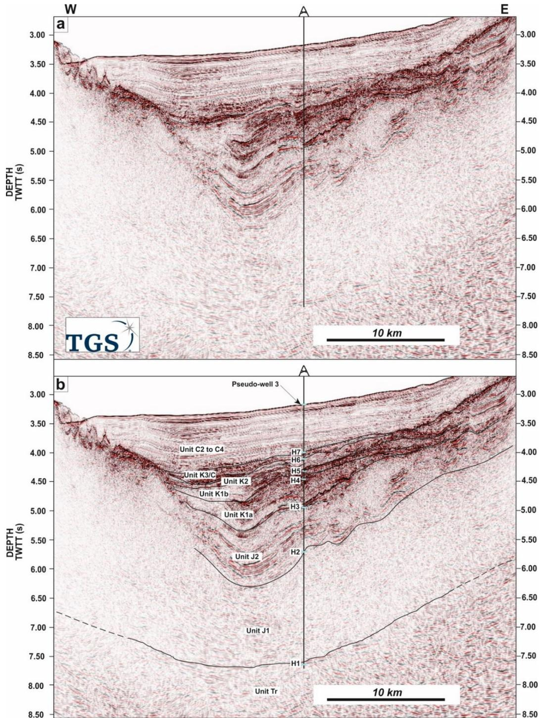
Figure 3.10: a) Uninterpreted E-W section, and b) corresponding interpretation of a seismic profile close to the northernmost part of the study area, into the Galicia Interior Basin. See Figure 3.1b for location. Note the absence of salt structures in this location and interpreted presence of thick salt. Location of pseudo-well 3 is also shown in the figure.
