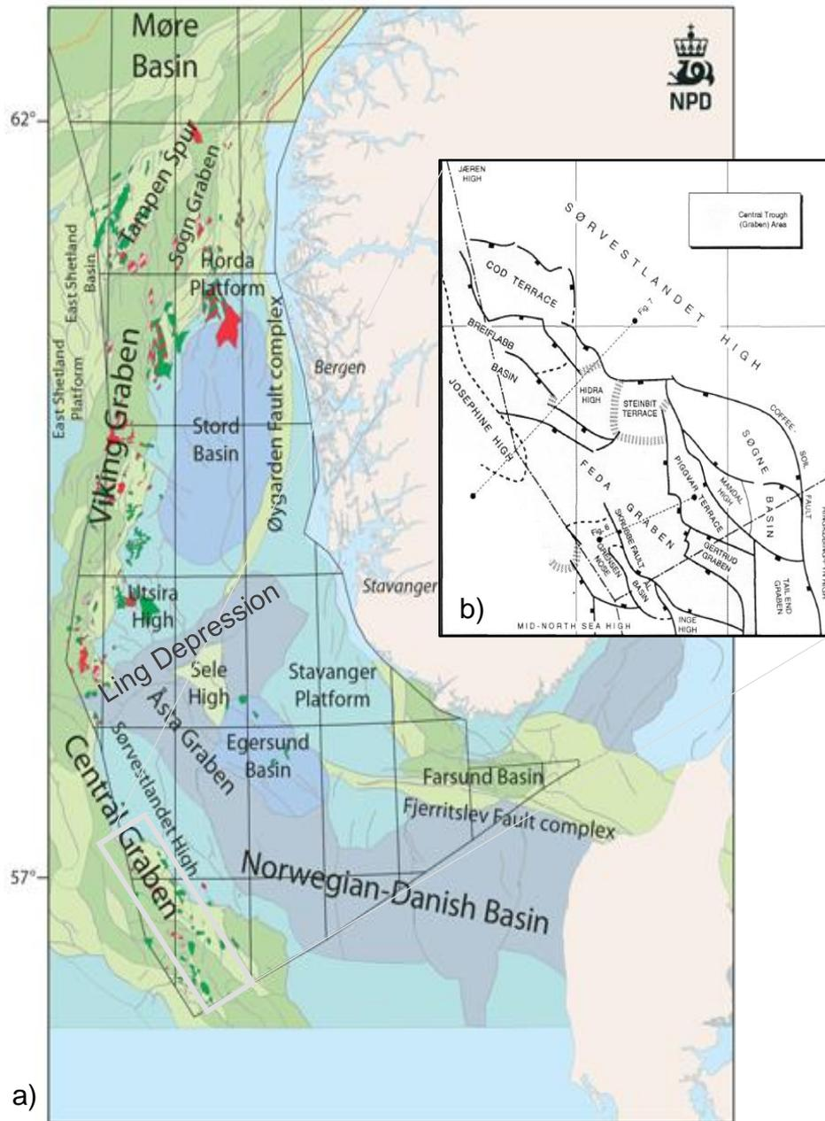
Figure 4.1: a) Map of Norwegian North Sea and geographical location showing main structural elements from NPD Norwegian Petroleum Directorate. b) Structural elements in the Central Graben active during the Jurassic-Early Cretaceous based on Gowers et al. (1993).
