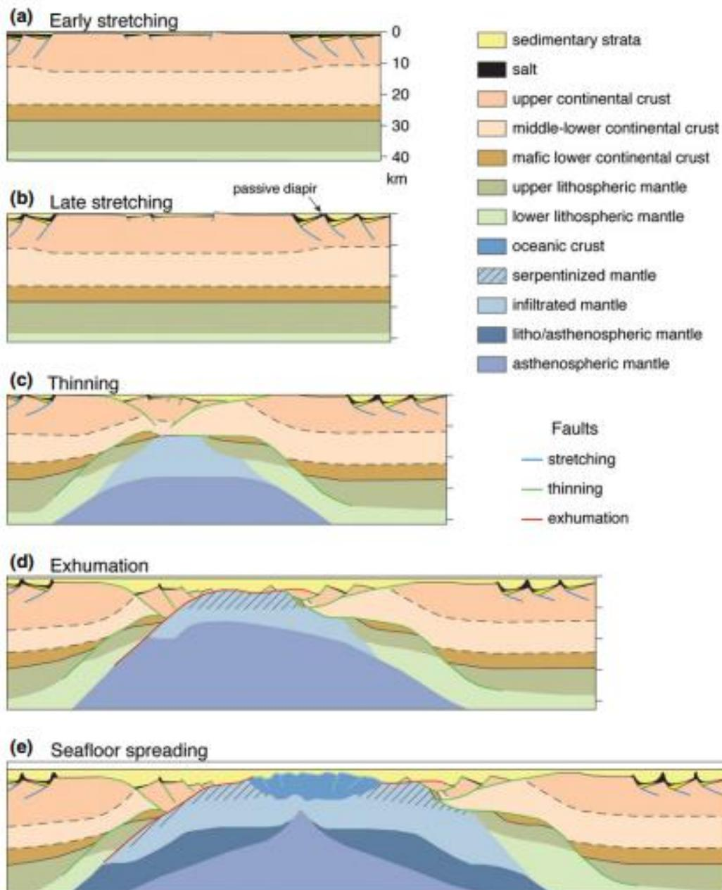
Figure 5.2. Model of syn-stretching salt basin using template modified from Peron-Pivodic and Manatschal (2009); a) early stretching stage with salt deposition controlled by active faults; b) late stretching stage with salt diapirism by ongoing thick-skinned extension; c) thinning stage with continued diapirism; d) exhumation stage with only minor continued salt-related deformation; and e) spreading stage showing salt concentrated in proximal areas. From Rowan et al. (2014).
