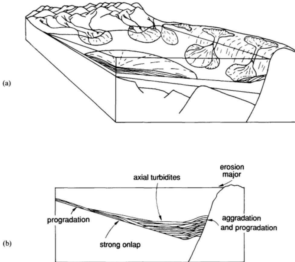
Figure 2.7: Immediate post-rift systems tract (a) generalised block diagram; (b) schematic cross section shows expansion and down-cutting of drainage basins, aggradation of facies through infillinf, prominent onlap surface and progradation of sediment into basin from transverse as well as longitudinal systems (Prosser, 1993).
