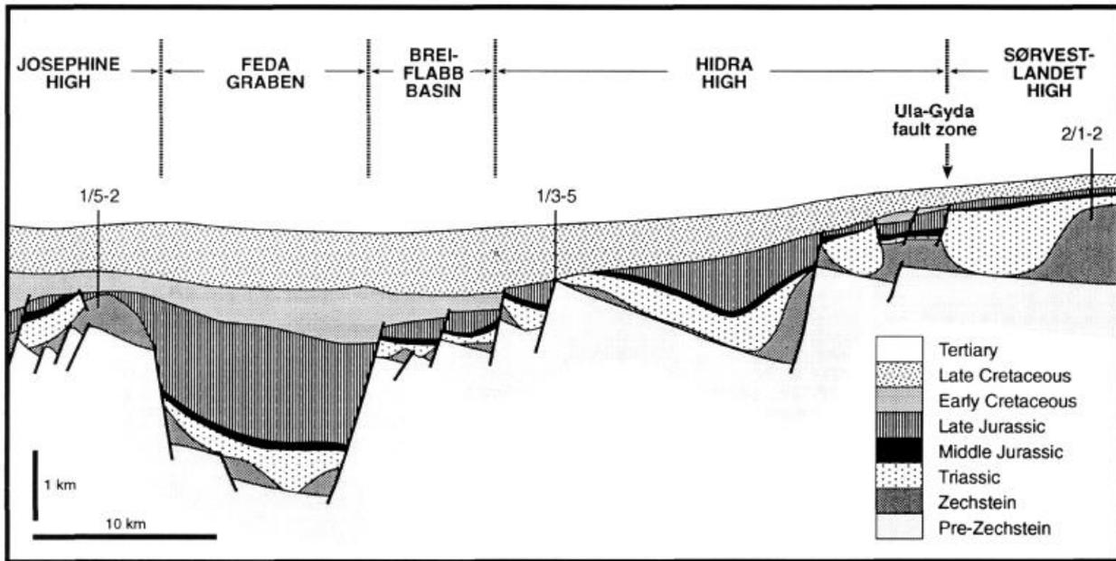
Figure 4.4: Regional cross section illustrating the broad structural styles and sedimentary packages observed from the Josephine to the Sorvestlandet High. Figure is modified from Gowers et al. (1993).
