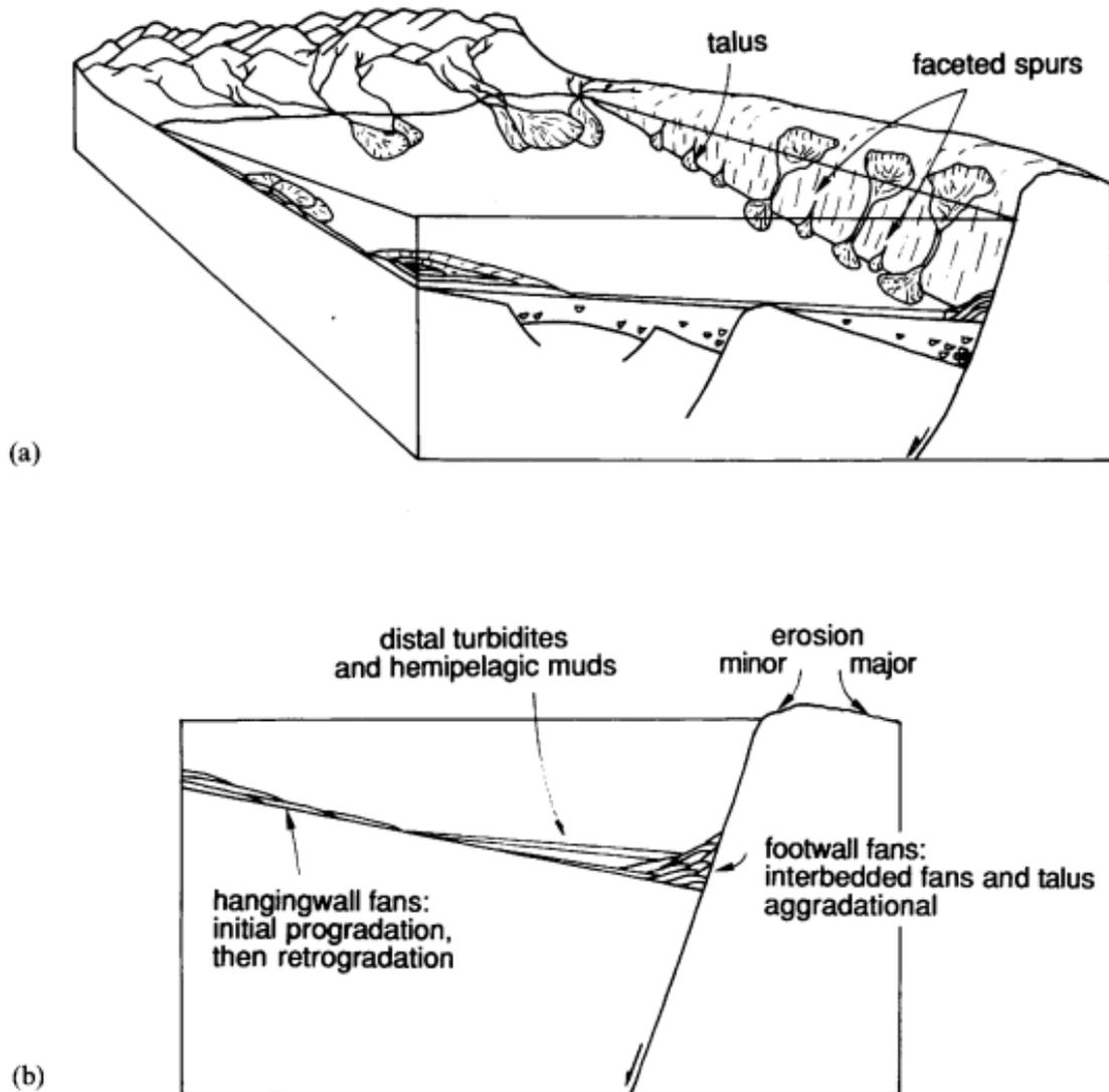
Figure 2.5: Rift climax systems tract (a) generalised block diagram shows increases area of deposition and small size of consequent drainage basins; (b) schematic cross section shows large relief on a single dominant fault plane (Prosser, 1993). Note this sketch represents late stage in climax of rifting when hangingwall has been transgressed and submerged.
