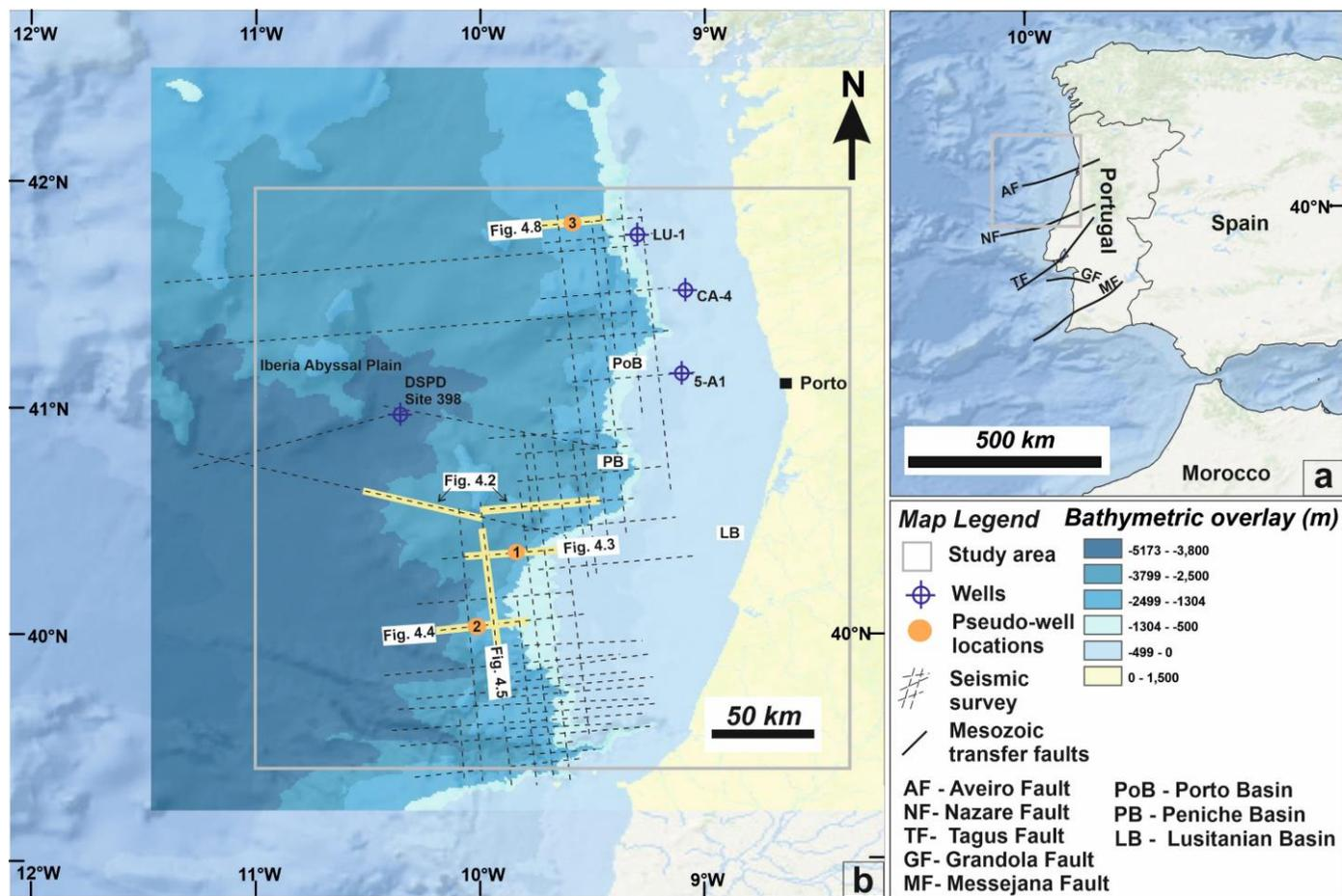
Figure 3.1: a) Map of the West Iberian margin and geographical location showing major transfer faults and the study area. b) Bathymetric map of study area depicting interpreted seismic grid with location of offshore industry and DSDP wells (Esri GEBCO 2019).
