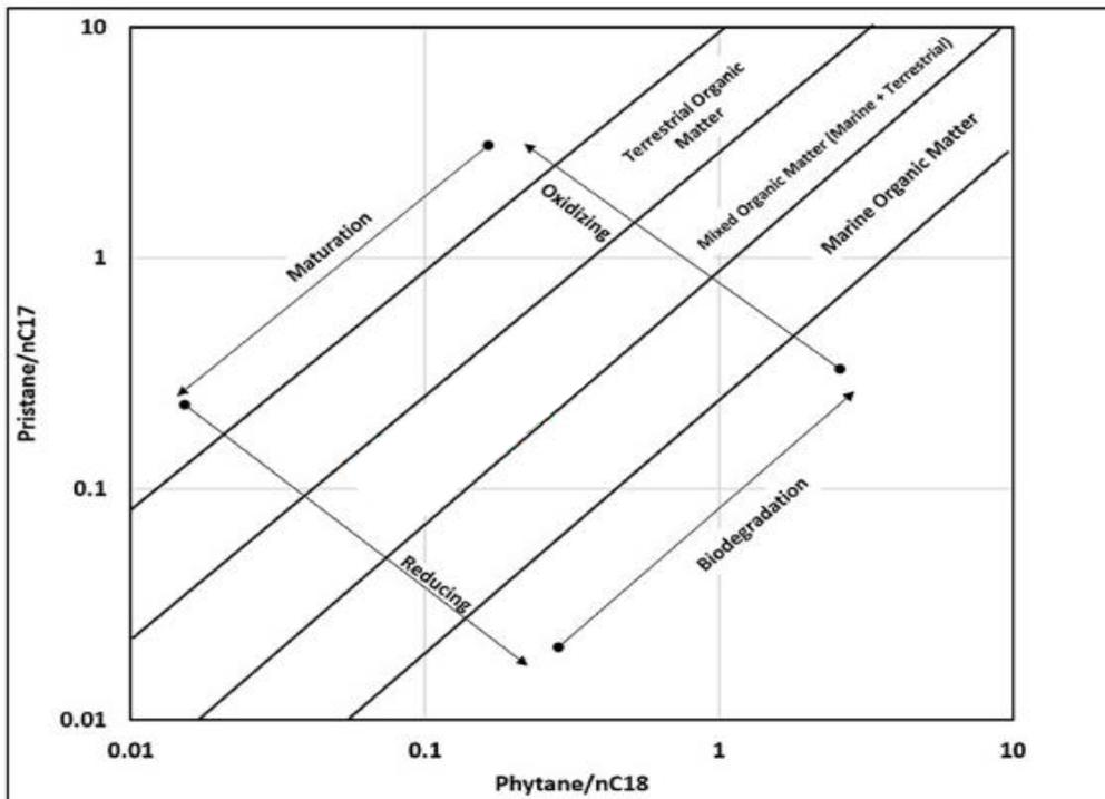
Figure 4.9: Classical Pr/nC17 versus Ph/nC18 plot (Author's own), providing information on depositional environment, kerogen type, and maturity level, where Pristane and Phytane represent isoprenoid hydrocarbons and nC17 and nC18 denote n-alkane hydrocarbons.
