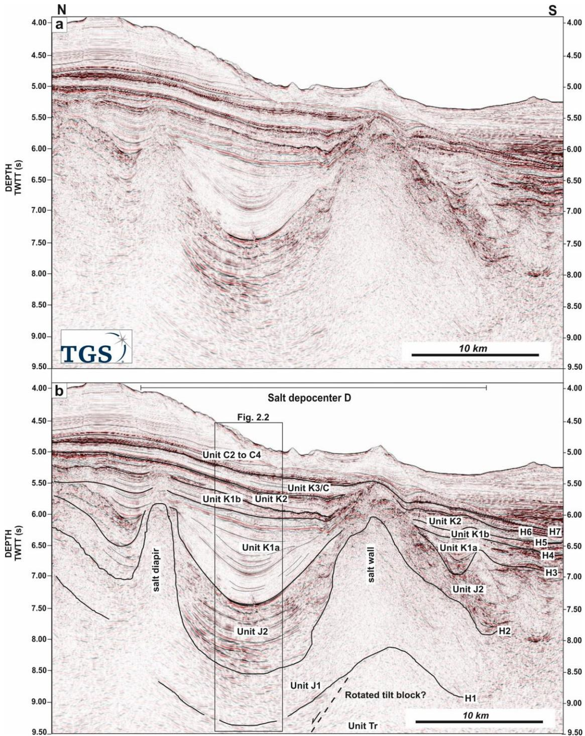
Figure 3.7: a) Uninterpreted section, and b) corresponding interpretation of a N-S seismic profile to the west of the Lusitanian Basin, on the continental slope. See Figure 3.1b for location. Note the presence of developed diapirs and the apparent formation of bowl-shaped depocentres during the Early Cretaceous rift 4 (Unit K1).
