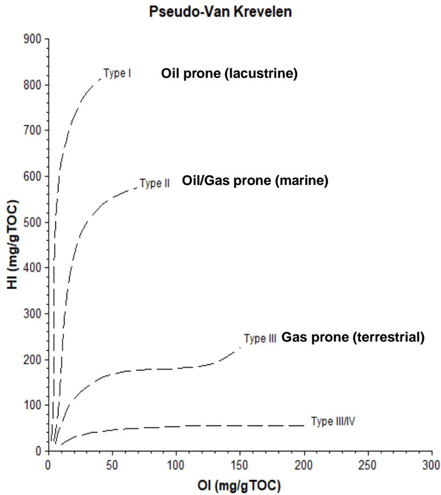
Figure 4.6: Pseudo Van Krevelen Diagram (Author's own) illustrating the cross-plot of the Oxygen Index (OI) against the Hydrogen Index (HI), depicting the typical ranges for Types I, II, and III kerogen.
