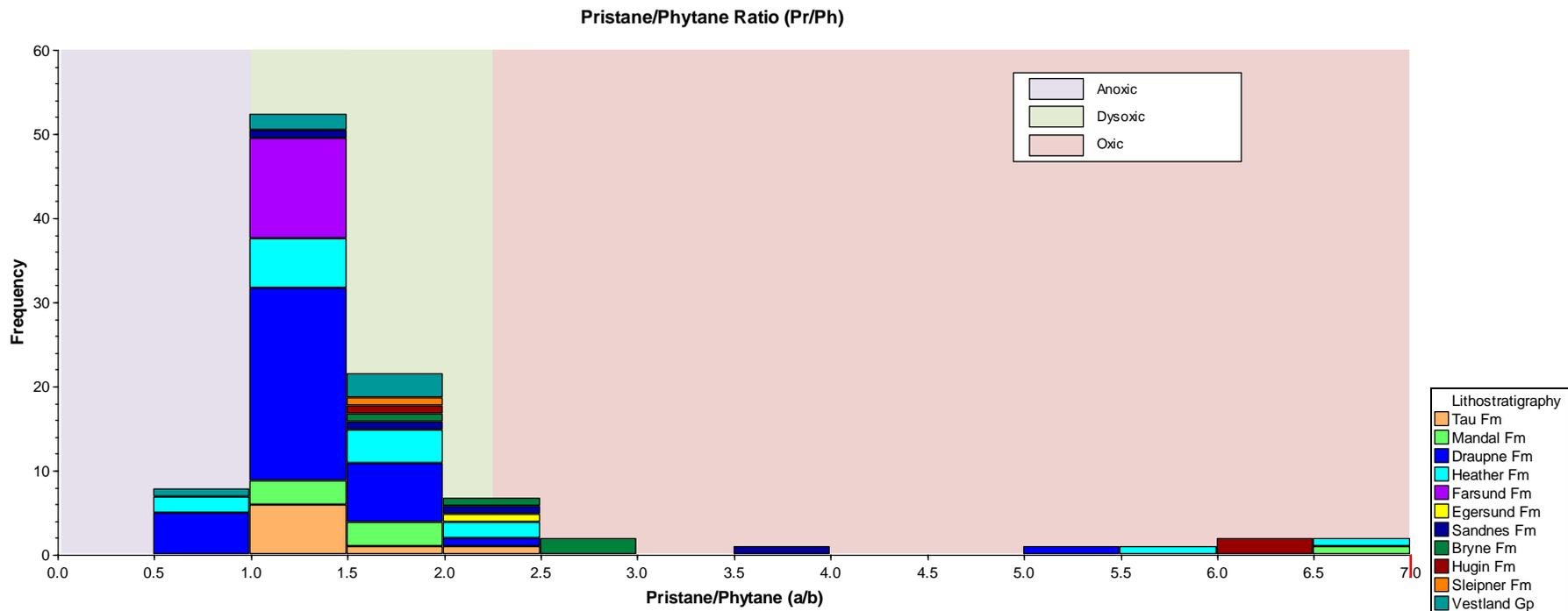
Figure 4.15: Pristane/Phytane ratio of samples inferred that the highest frequency of the source rocks samples were deposited mainly in dysoxic environments, whilst others were likely deposited in anoxic and oxidic environments, respectively.
