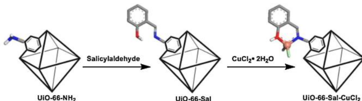
Figure 9: Lu and co-workers' method to immobilising a homogeneous Cu catalyst on UiO-66-NH 2 . 86
