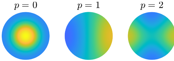
Fig. 7 Illustrations of equation (43) for p = 0, 1 and 2 . \rho \in [0, R] and the k > 0 value depends on p and is defined by B'_p(kR) = 0 , see text, Table 1 and Fig. 6a for details. The colour axis in all cases is fixed to be blue at -1 and yellow at 1 (Color figure online)
